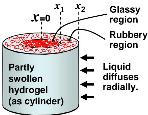
**Fig. 10.** Model of partly swollen hydrogel as a segment of an infinite cylinder, to enable derivation of a non-Fickian diffusion-based rate of absorbency. The model is based on an assumed much greater diffusion rate within a rubbery (already swollen) layer.
