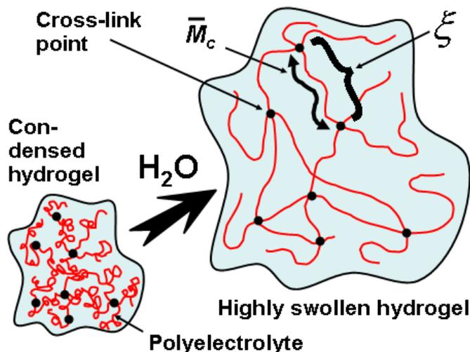
**Fig. 4.** Representation of a hydrogel in its somewhat condensed (left) and highly swollen (right) states. Solid dots indicate cross-linked points of the polyelectrolyte chains (shown as coiled or wavy lines). The characteristic molecular weight of segments between crosslinks ( $\bar{M}_c$ ) and the correlation distance between crosslink points ( $\xi$ ) are illustrated by considering one segment.
