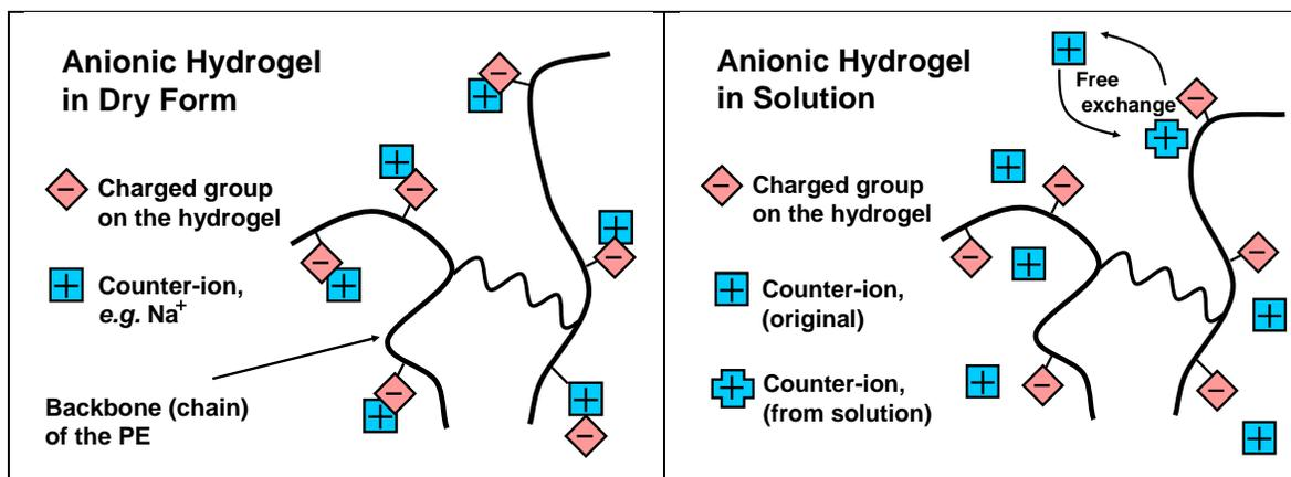
**Fig. 3.** Illustration of increased disorder and freedom of motion of a counter-ion (e.g. sodium) in a typical hydrogel that contains acid groups (e.g. carboxylate). **Left:** Dry form as sodium salt of polycarboxylate hydrogel; **Right:** Water-swollen form, in which the counter-ions are free to exchange with each other, to diffuse within the field of electrostatic forces, and also for the polyelectrolyte chain segments to undergo some constrained motion.
