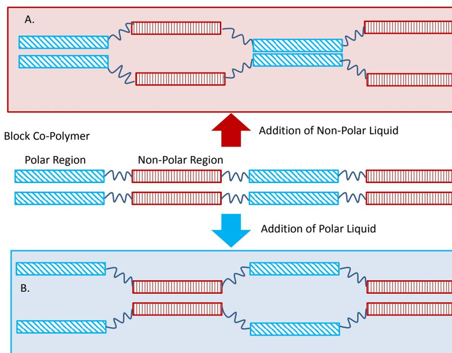
**Fig. 12.** Block co-polymer containing both polar and non-polar domains. **A:** Immersion of material into non-polar solvent causes the non-polar regions to swell and absorb liquid, while polar regions prevent the dissolution of the polymer. **B:** Immersion of material into polar solvent causes the polar regions to swell and absorb liquid, while non-polar regions prevent the dissolution of the polymer.
