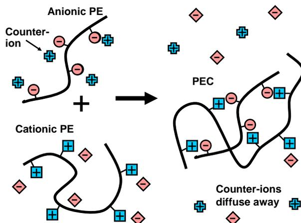
**Fig. 7.** Mechanism of polyelectrolyte complex (PEC) formation in which ion pairing between bound groups on the respected polyacid and polybase chains make it possible for the monomeric counter-ions to diffuse away, with a large increase in entropy of the system.
