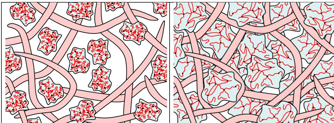
**Fig. 5.** Illustration of the concept that a network of macroscopic cellulosic fibers in an absorbent product might tend to constrain the swelling of hydrogel particles. **Left:** Representation of dry condition; **Right:** Swollen condition
