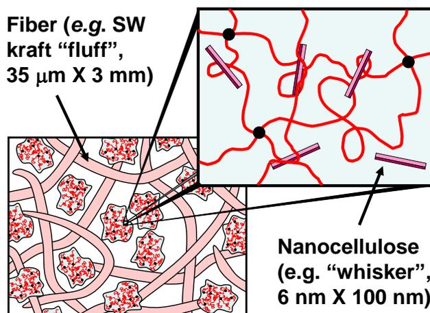
**Fig. 6.** Illustration emphasizing the great size difference between fluff pulp fibers vs. cellulosic nanocrystal, a difference that suggests that their roles with respect to reinforcement, crosslinking, or other effects might also be different
