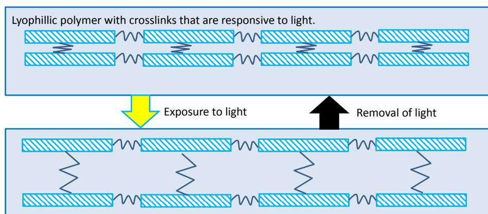
**Fig. 13.** Schematic view of a lyophilic polymer crosslinked with a light-sensitive polymer. Upon exposure to light, the crosslink polymer conformation changes, allowing for the absorbent to take up a large fraction of liquid. If this is a reversible process, then removing the stimulus could result in the expulsion of the liquid.
