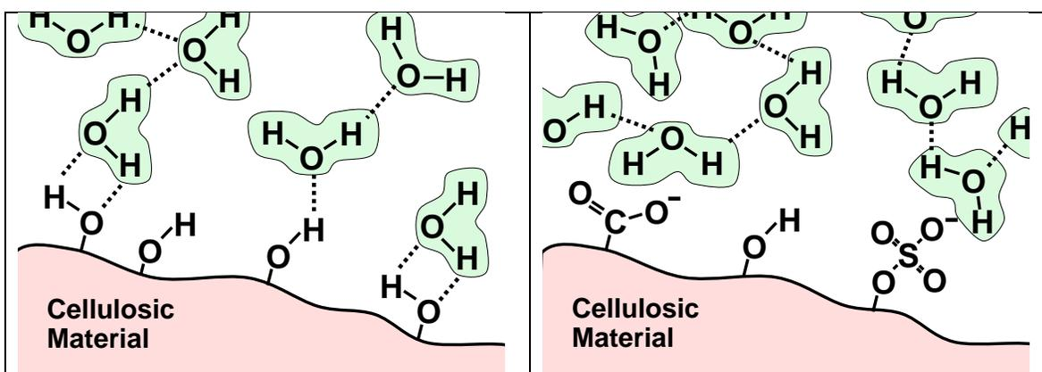
**Fig. 2.** Representation of hydrogen bonding among the molecules of liquid water and also associated with hydrophilic groups. **Left:** Hydrogen bonding associated with hydroxyl groups bound to a substrate. **Right:** Interaction and orientation of polar H<sub>2</sub>O molecules with ionized groups such as carboxylate or sulphonate groups, all associated with the transient hydrogen bonded structure of liquid water
