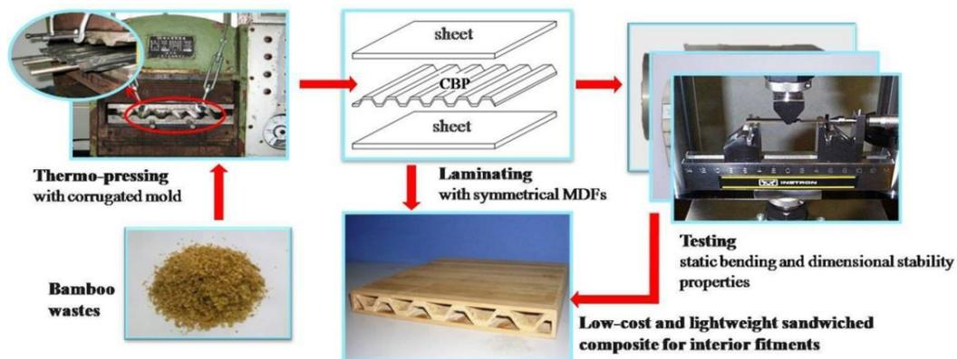
Fig. 1. Preparation process of sandwiched panel
