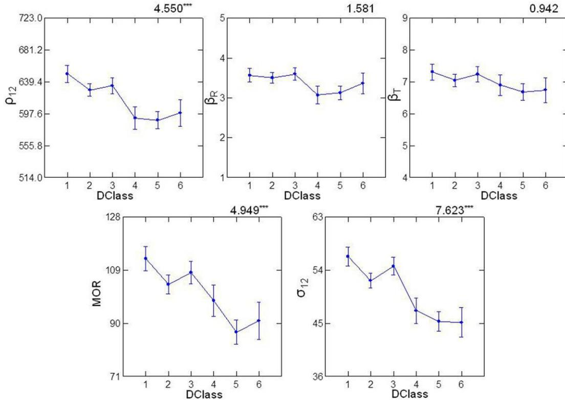
**Fig. 4.** ANOVA analysis of the effect of diameter class on physical and mechanical properties of whole trees aged 25–30 years at Site A
