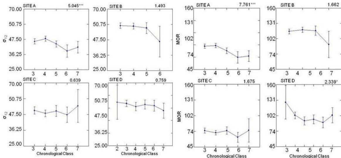
**Fig. 3.** ANOVA analysis of the effect of chronological class on compressive strength and MOR. The numbers above the graphs are F values with significant probability: \*  $p < 0.05$ , \*\*  $p < 0.01$ , \*\*\*  $p < 0.001$ .
