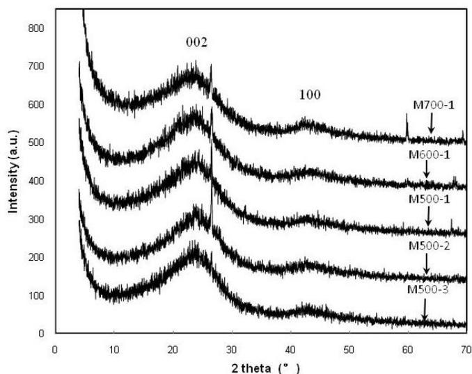
Fig. 3. XRD diffraction patterns of active carbon monoliths
