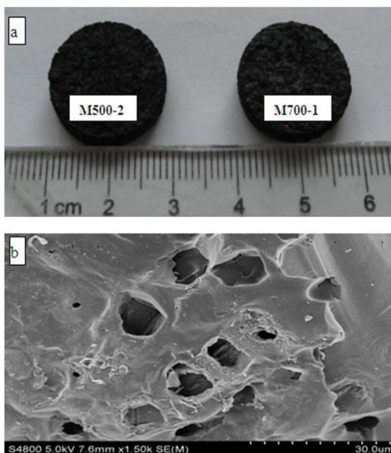
**Fig. 1.** Morphology of active carbon monoliths: (a) photos of active carbon monoliths, (b) SEM image for M700-1 at a magnification of 1500
