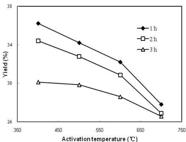
Fig. 2. Yield of active carbon monoliths
