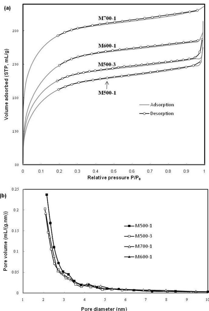
**Fig. 4.** (a) Adsorption/desorption isotherms and (b) pore size distributions of active carbon monoliths
