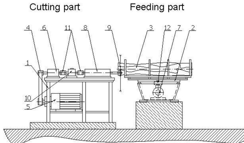
**Fig. 2.** Illustration of the experimental measuring device: 1 - a working table, 2 - a sliding line, 3 - a trunk of round timber, 4 - belts to drive the circular saw, 5 - an electric engine to drive the circular saw, 6 - a bearing cover, 7 - an electric engine to push the material to the cut, 8 - a spindle head of a circular saw, 9 - a circular saw, 10 - a T20WN recording device for torque and rotational speed, 11 - a GFL-28 clutch, 12 - an S2 force recorder
