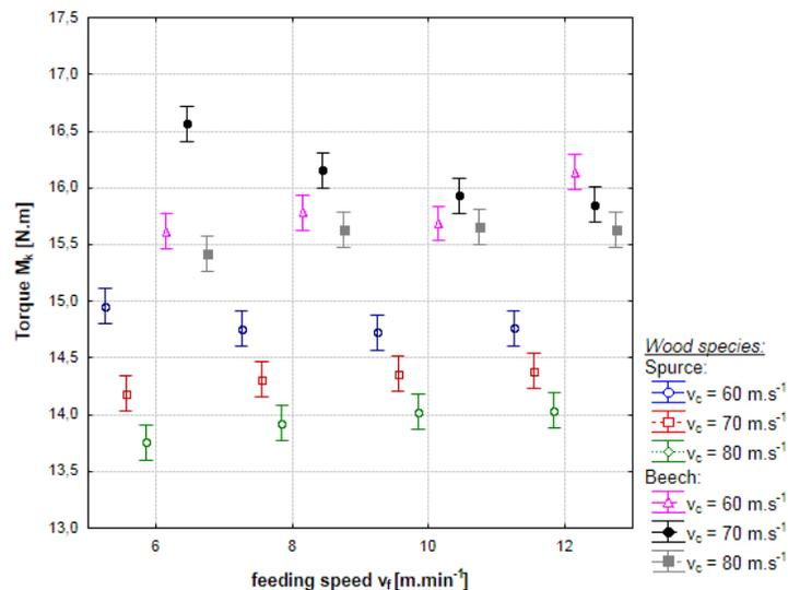
**Fig. 7.** The influence of feeding speed  $v_f$  on torque  $M_k$  for different wood species
