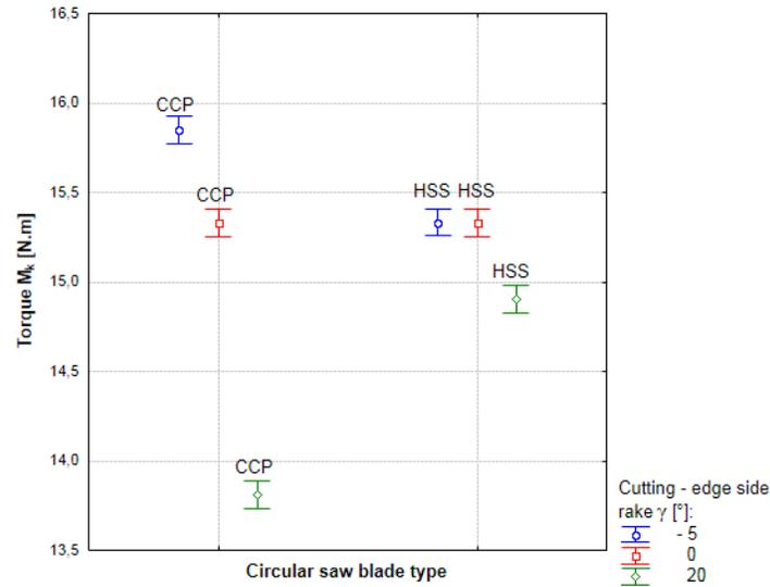
**Fig. 10.** The influence of circular saw type on torque for different cutting-edge side rakes
