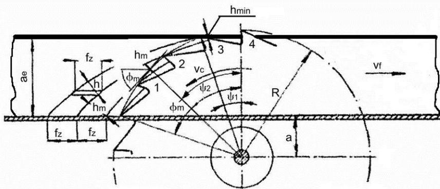
**Fig. 1.** Illustration of a circular saw cutting wood:  $f_z$  – feed per one tooth [ $\text{m}\cdot\text{s}^{-1}$ ],  $a_e$  – cutting height [m],  $v_f$  – feeding speed [ $\text{m}\cdot\text{s}^{-1}$ ],  $v_c$  – cutting speed [ $\text{m}\cdot\text{s}^{-1}$ ],  $\psi_1$  – incoming angle of a circular saw [°],  $\psi_2$  – outgoing angle of a circular saw [°],  $\phi_m$  – mean angle of cutting fibres [°],  $h_m$  – mean thickness of a chip [mm]
