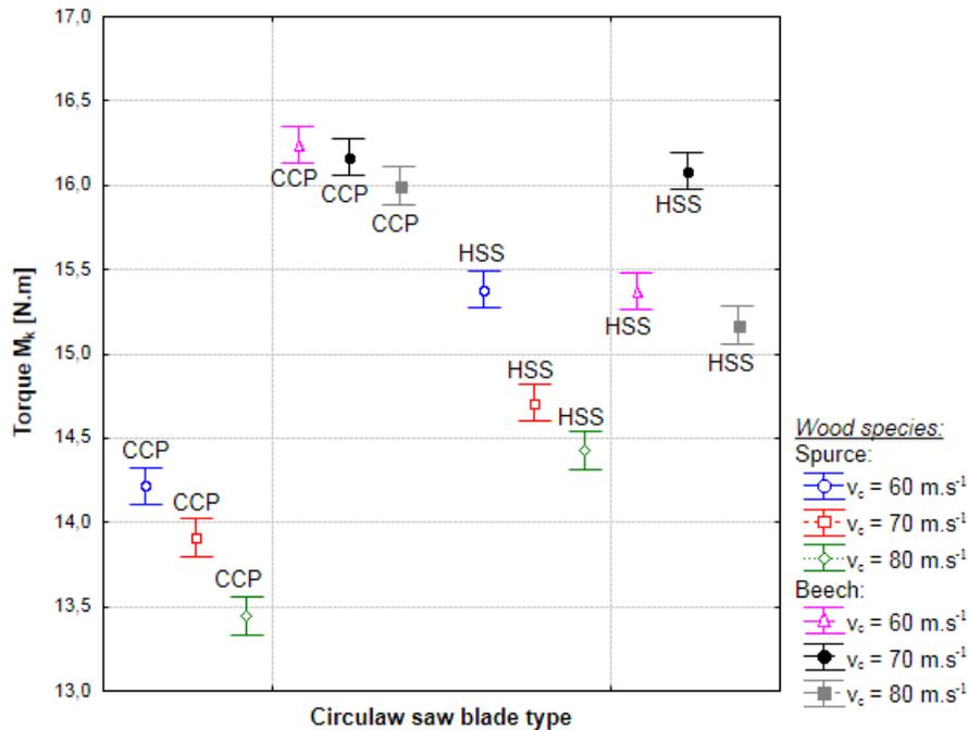
Fig. 9. The influence of circular saw type on torque  $M_k$  for different wood species
