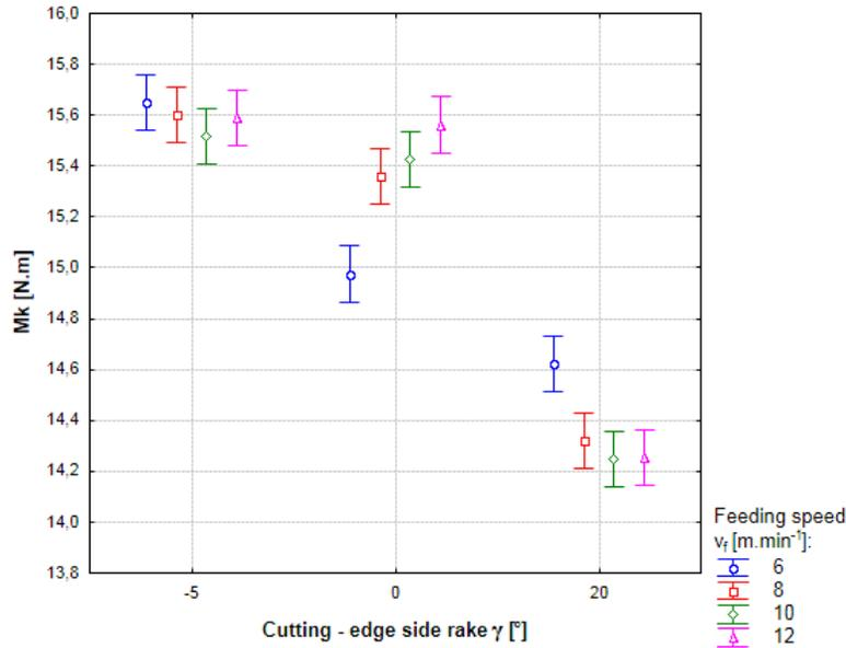
Fig. 8. The influence of cutting-edge side rake on torque  $M_k$  for varying feeding speeds  $v_f$
