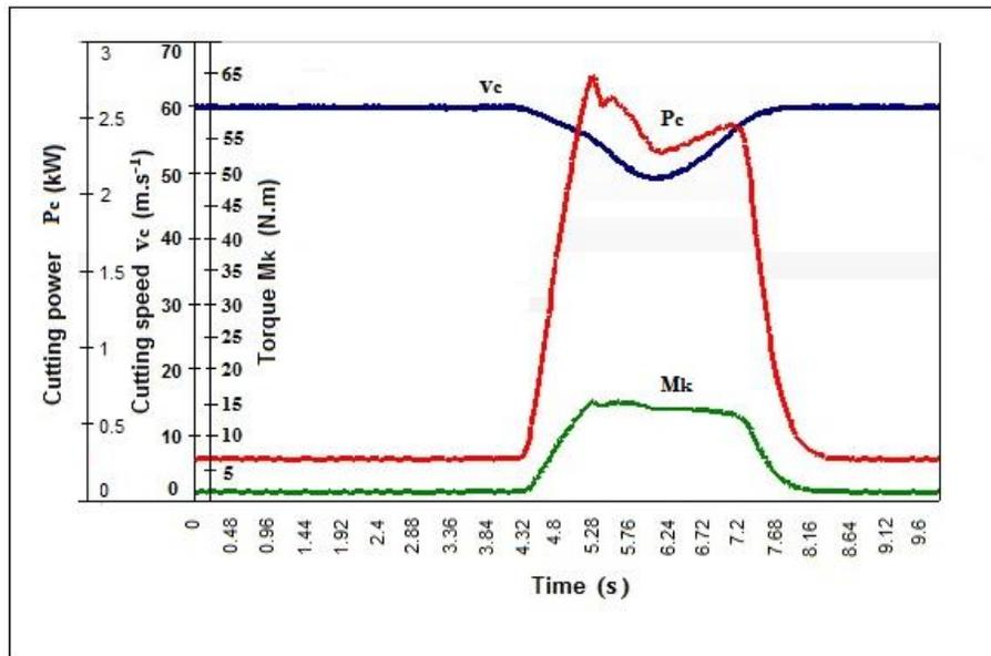
**Fig. 5.** The course of  $M_k$  during the crosscutting process of beech sawn by a circular saw made of cemented carbide plates with a cutting-edge side rake of  $20^\circ$
