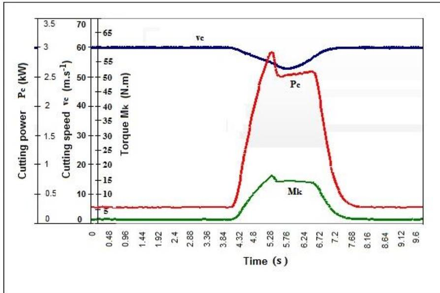
**Fig. 6.** The course of  $M_k$  during the crosscutting process of beech sawn by a circular saw made of high speed steel with a cutting-edge side rake of  $20^\circ$
