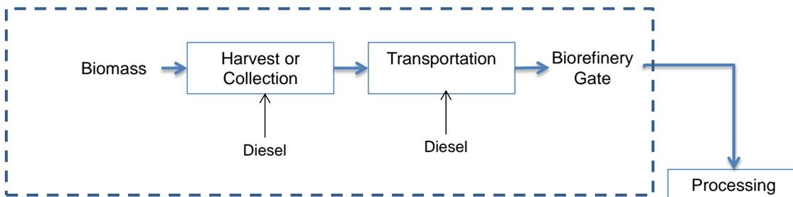
Fig. 4. Production stages and system boundary of forest residue collection and delivery
