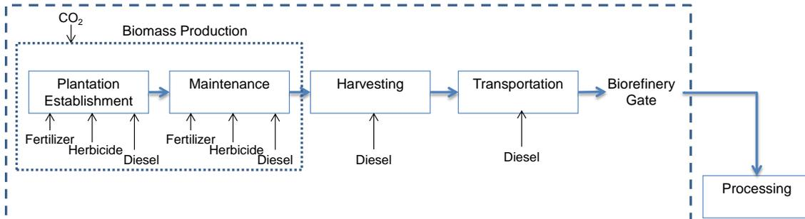
Fig. 3. Production stages and system boundary of forestry biomass production and delivery
