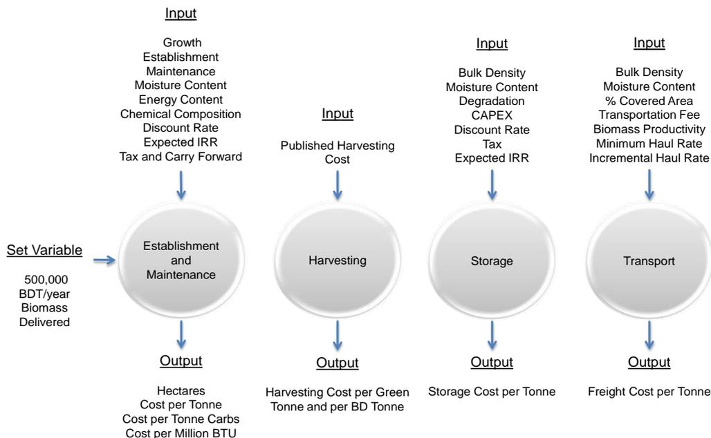
**Fig. 2.** Inputs and outputs of the biomass supply chain model
