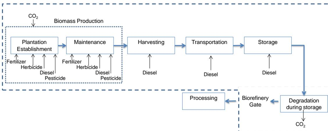
**Fig. 5.** Production stages and system boundary of agricultural biomass production and delivery; note: degradation emissions and CO<sub>2</sub> uptake during growth are shown separately for clarification
