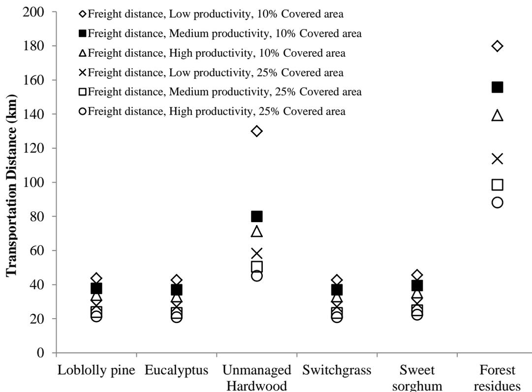
**Fig. 6.** Maximum freight transportation distances from biomass source to processing facility, assuming 500,000 BDT/year (453,592 metric tonnes/year), feedstock-specific productivity, and covered area values as indicated. All transportation distances include a tortuosity factor of 1.31 km transported per linear km of distance from point of biomass harvest to biorefinery (Ravula 2007).
