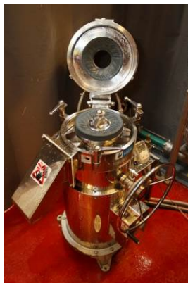
Fig. 1. Masuko Sangyo ultrafine friction grinder (MKZA10-15J) equipped with fine MKGA10-80 stones made of aluminum oxide and resins
