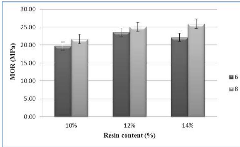
**Fig. 1.** Modulus of rupture of samples manufactured with different refining conditions (pressure 6 and 8 bar) and resin contents
