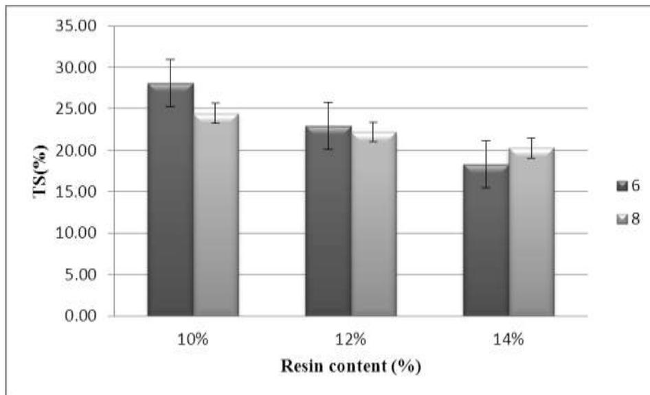
**Fig. 5.** Thickness swelling of samples manufactured with different refining conditions (pressure 6 and 8 bar) and resin contents
