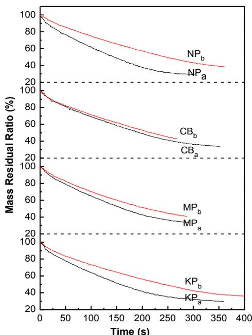
**Fig. 4.** Mass residual ratios of the specimens with 30 mm thickness from the four types of raw materials at the levels of 500 mL (with label a) and 900 mL (with label b) Si-Al compounds at 50 kW/m<sup>2</sup>. KP, MP, CB, and NP stand for kraft pulp, mechanical pulp, cardboard, and newspaper, respectively.
