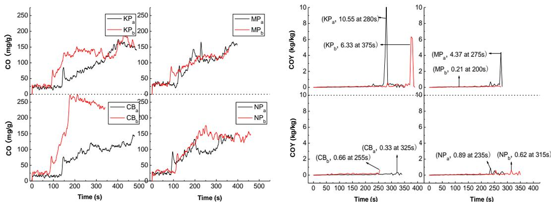
**Fig. 6.** CO concentration (left) and CO yield (COY, right) profiles of the specimens with 30 mm thickness from the four types of raw materials at the levels of 500 mL (with label a) and 900 mL (with label b) Si-Al compounds at 50 kW/m<sup>2</sup>. KP, MP, CB, and NP stand for kraft pulp, mechanical pulp, cardboard, and newspaper, respectively.
