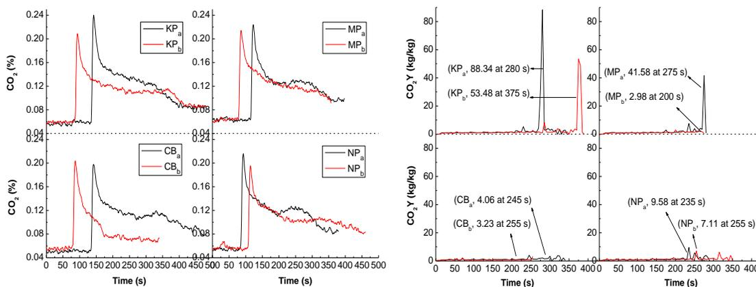
**Fig. 7.** CO<sub>2</sub> concentration (left) and the yield (CO<sub>2</sub>Y, right) profiles of the specimens with 30 mm thickness from the four types of raw materials at the levels of 500 mL (with label a) and 900 mL (with label b) Si-Al compounds at 50 kW/m<sup>2</sup>. KP, MP, CB, and NP stand for kraft pulp, mechanical pulp, cardboard, and newspaper, respectively.
