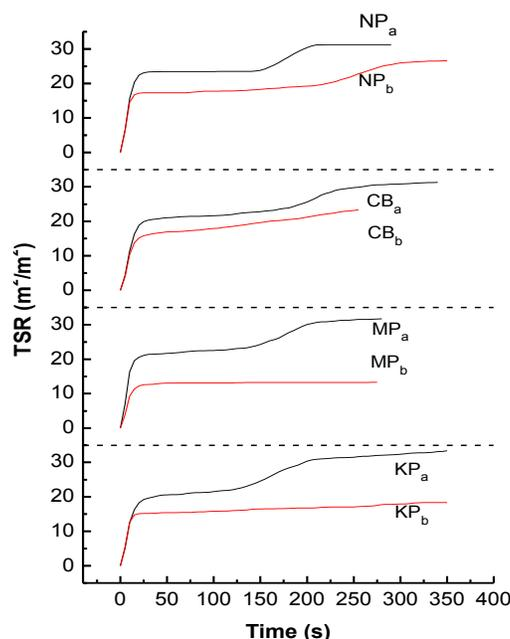
**Fig. 5.** TSR profiles of the specimens with 30 mm thickness from the four types of raw materials at the levels of 500 mL (with label a) and 900 mL (with label b) Si-Al compounds at 50 kW/m<sup>2</sup>. KP, MP, CB, and NP stand for kraft pulp, mechanical pulp, cardboard, and newspaper, respectively.
