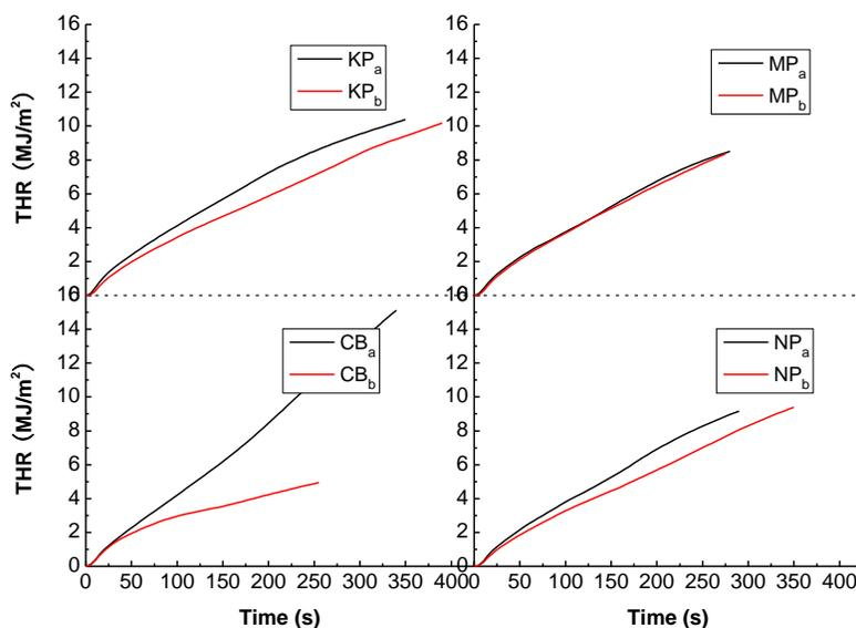
**Fig. 3.** THR profiles of the specimens with 30 mm thickness from the four types of raw materials at the levels of 500 mL (with label a) and 900 mL (with label b) Si-Al compounds at  $50 \text{ kW/m}^2$ . KP, MP, CB, and NP stand for kraft pulp, mechanical pulp, cardboard, and newspaper, respectively.
