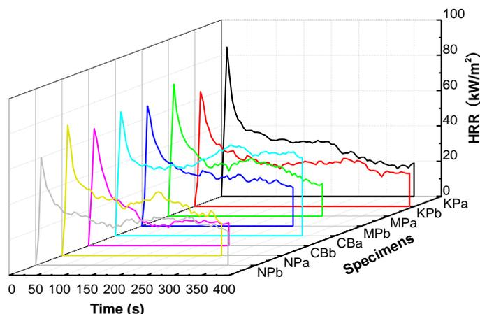
**Fig. 2.** HRR profiles of the specimens with 30 mm thickness from four types of raw materials at the levels of 500 mL (with label a) and 900 mL (with label b) Si-Al compounds at 50 kW/m<sup>2</sup>. KP, MP, CB, and NP stand for kraft pulp, mechanical pulp, cardboard, and newspaper, respectively.
