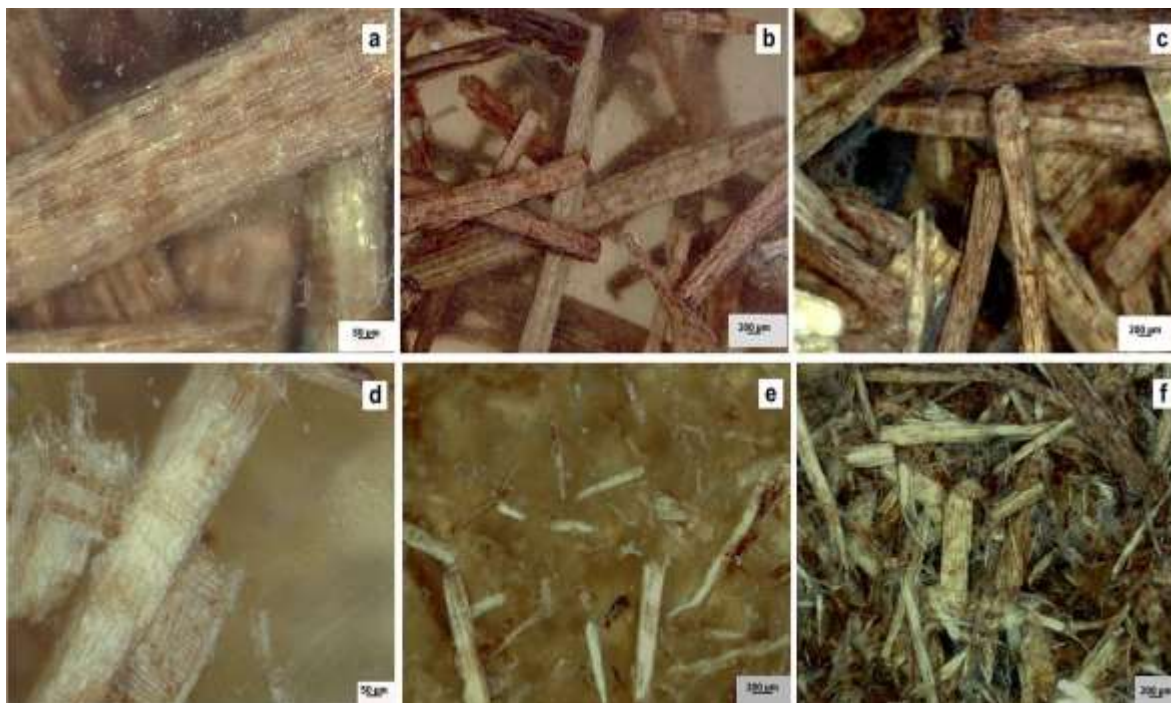
Fig. 1. Micrographs of bio-composites with eucalyptus particle sizes of 8 mm (a-c) and 4 mm (d-f) and amounts of 5% (b, e) and 20% (c, f). Micrographs (a) and (d) correspond to enlargements of samples (b) and (e), respectively.
