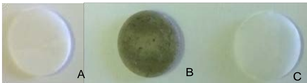
Fig. 6. Pictures of translucent disks used for FTIR analysis: A- potassium bromide pellet (used as blank); B- biosurfactant pellet from Beta vulgaris ; C- pellet of standard surfactin from Sigma Aldrich
