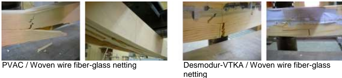
Fig. 10. Examples of experimental results of bending resistance parallel to the glue line
