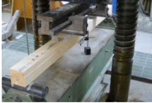
Fig. 6. Four points bending test
