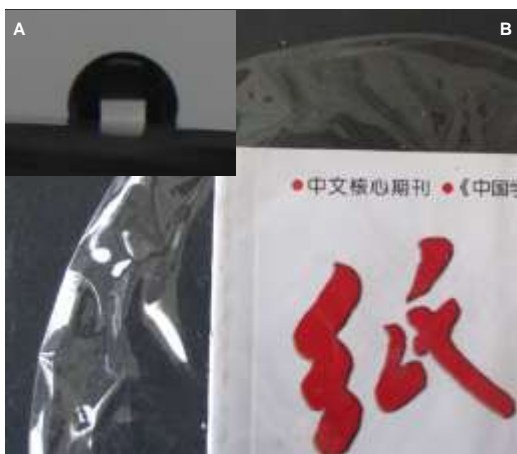
Fig. 6. Contact angle of cellulose ester film with water (A) and photograph of cellulose ester film (B)
