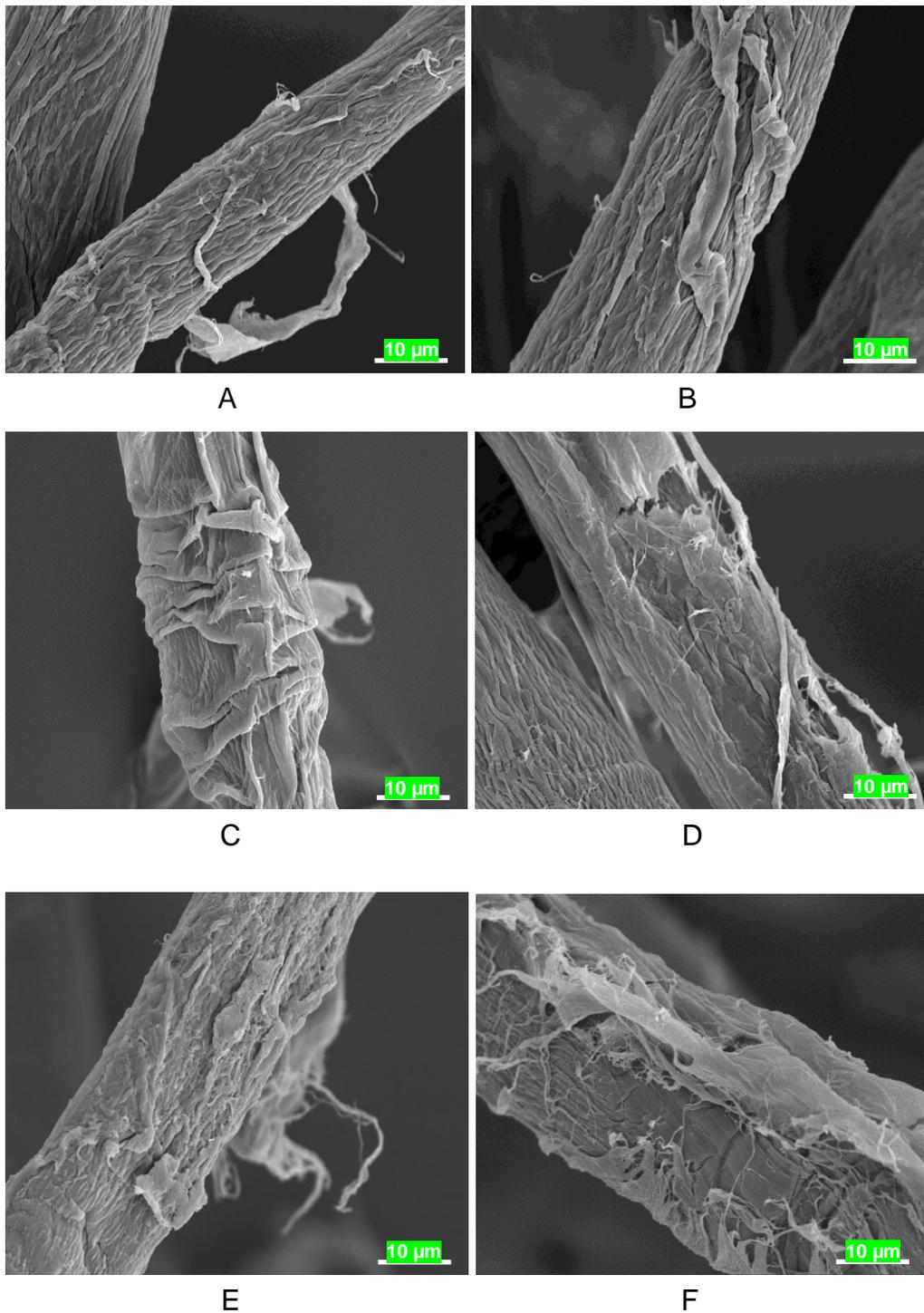
**Fig. 2.** Pulp morphology at air drying and freezing drying conditions. (A and B original pulp; C and D beating at 5000 revolutions; E and F beating at 10000 revolutions. A, C, E were with air drying; B, D, F were with freezing drying)
