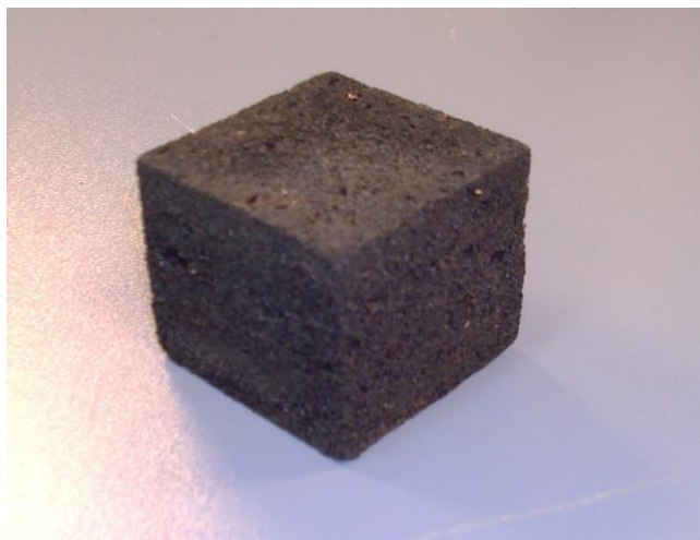
Fig. 5. Picture of a spruce tannin-based foam with the reference composition
