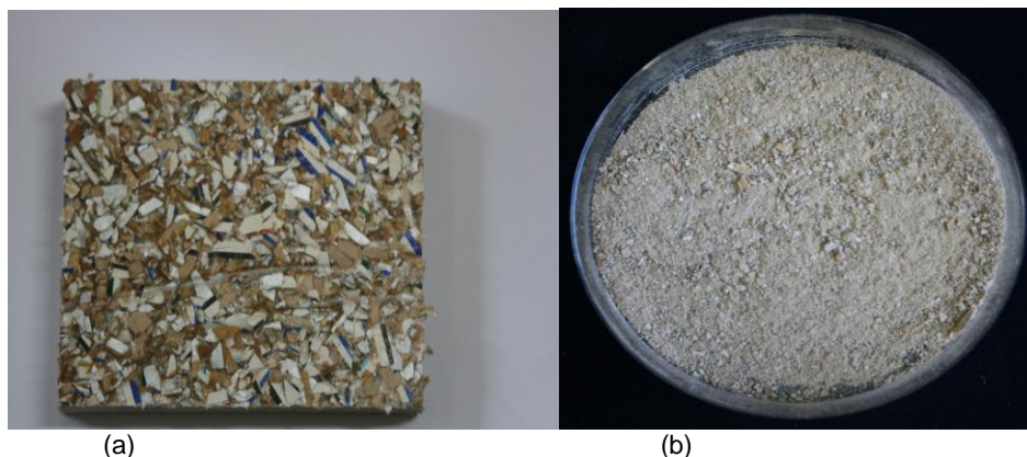
Fig. 1. (a) Tetra pak® panel specimen; (b) Ground material from panels
