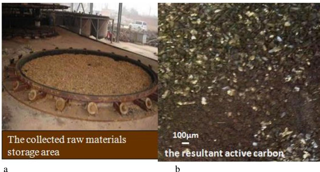
Fig. 1. a: Bitter almond shell powder; b: the resultant activated carbon
