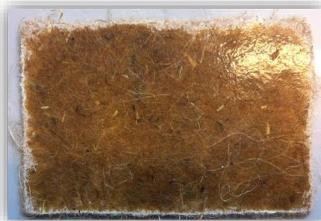
**Fig. 2.** A representative image showing the morphological characters of the hemp fibre-reinforced wheat gluten samples
