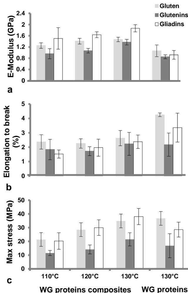
**Fig. 5.** Effect of temperature and protein type on (a) E-Modulus, (b) elongation at break and (c) maximum stress of the hemp fibre-reinforced proteins (WG, glutenin, and gliadin separately) compared with protein samples compression moulded without hemp fibres. Bars represent the standard deviation. For fibre content in each of the samples, (Table 1).
