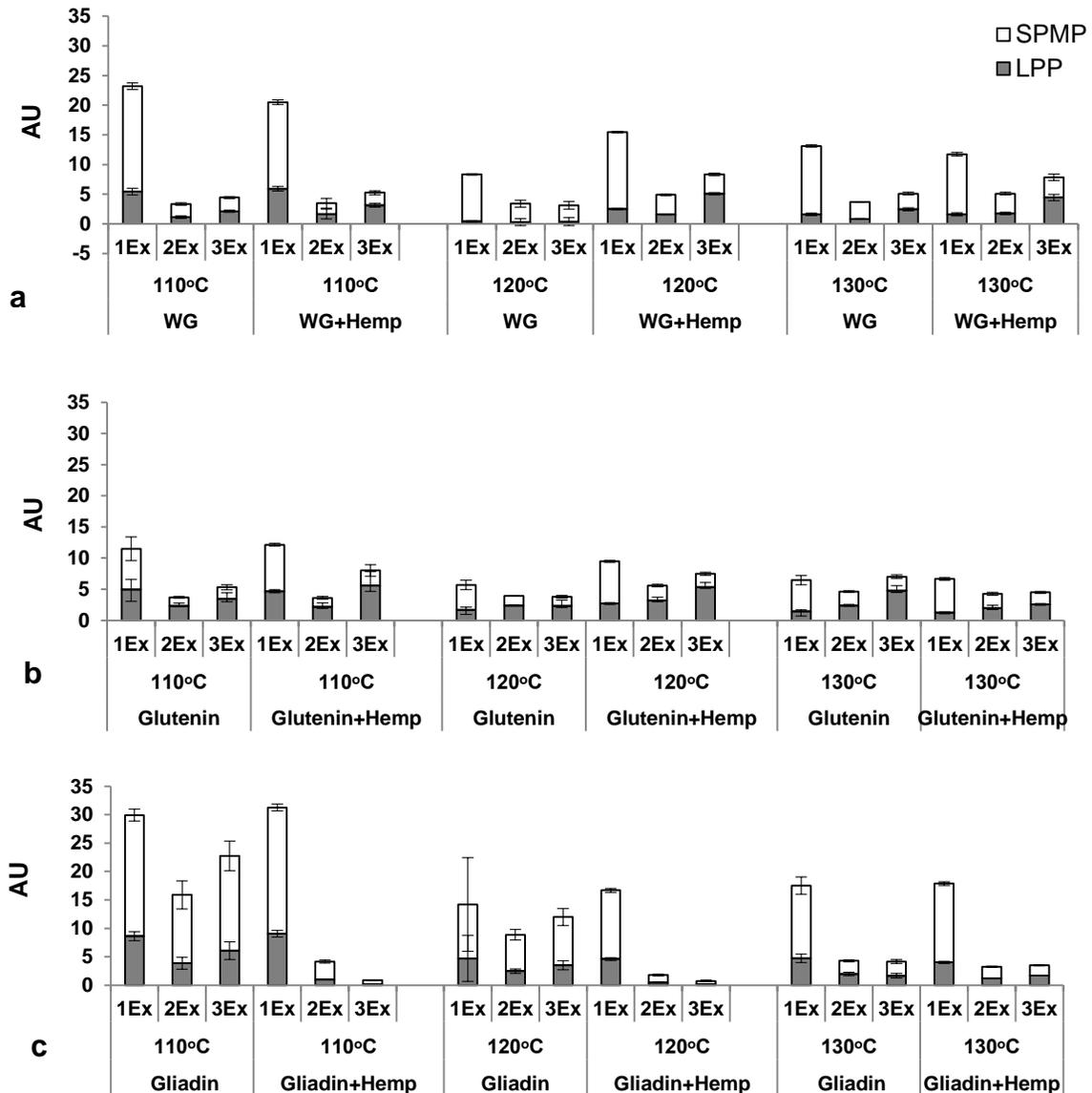
**Fig. 3.** Effect of temperature on the polymerisation of small polymeric and monomeric proteins (SPMP) and large polymeric proteins (LPP) in (a) compression moulded WG and hemp fibre-reinforced WG composites, (b) compression moulded glutenin and hemp fibre-reinforced glutenin composites, and (c) compression moulded gliadin and hemp fibre-reinforced gliadin composites. Bars represent the standard deviation.
