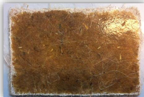
**Fig. 2.** A representative image showing the morphological characters of the hemp fibre-reinforced wheat gluten samples
