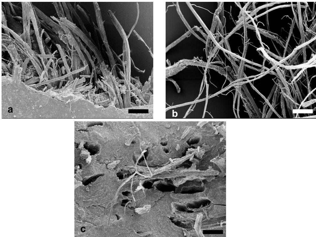
**Fig. 6.** SEM micrographs showing fibre pull-out in (a) hemp fibre-reinforced wheat gluten, compression moulded at 130 °C , (b) raw hemp fibres, and (c) clean holes after fibre pull-out (bars correspond to 100 µm for a, b, and c)
