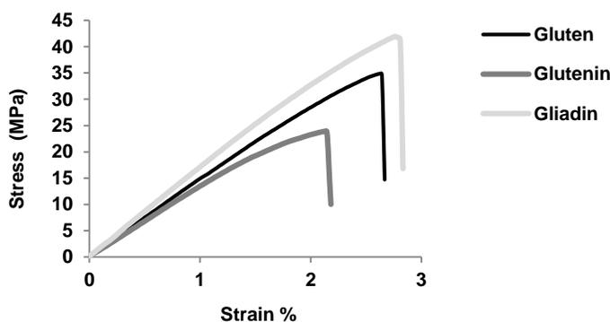
**Fig. 4.** Representative tensile behaviour of hemp fibre-reinforced WG, glutenin and gliadin composites (130 °C).
