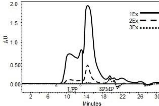
**Fig. 1.** A representative chromatogram showing extraction and separation of the proteins in compression moulded samples during the first (1Ex), second (2Ex), and third (3Ex) extractions.
