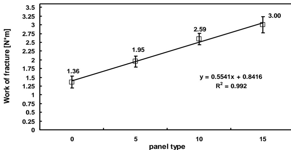
**Fig. 7.** Dependence of work of fracture of the investigated panels on RCF content
