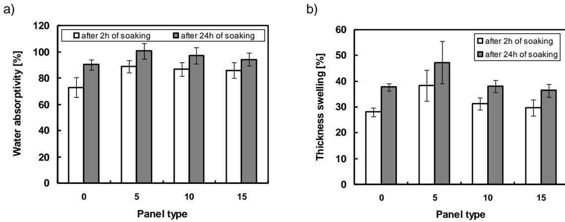
Fig. 4. Physical properties of investigated panels: water absorptivity a) and thickness swelling b)
