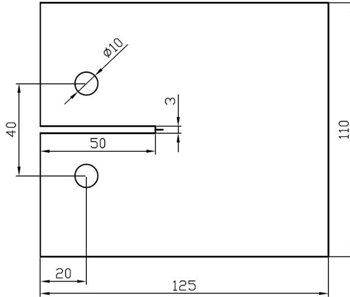
**Fig. 1.** Shape and dimensions (in millimeters) of the samples used to work of fracture measurement (based on Matsumoto and Nairn 2012)
