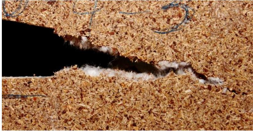
**Fig. 6.** Example of crack of the panel with 10% RCF content (the “bridging effect”)
