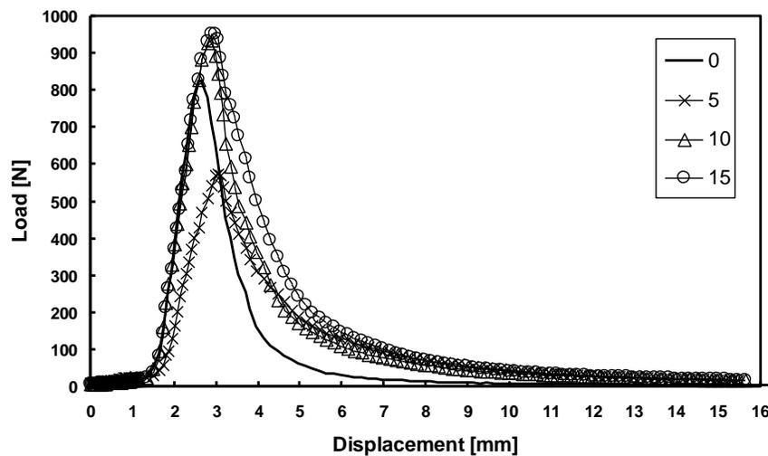
Fig. 4. The influence of regenerated cellulose fibers content in the panels on load-displacement curves
