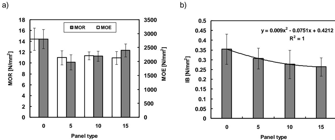
Fig. 3. Modulus of rupture a), modulus of elasticity a) and internal bond b) of tested composites
