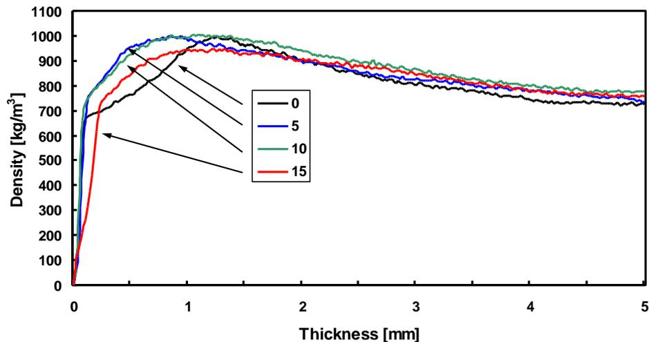
**Fig. 2.** Density profiles of the tested panels (half of thickness)
