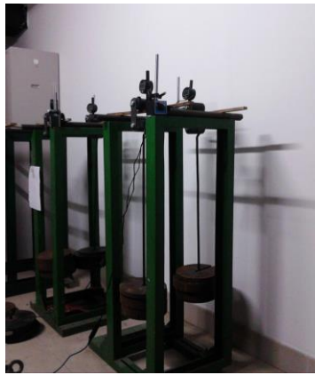
Fig. 2. Long term creep fixture used in the bending creep tests of specimens
