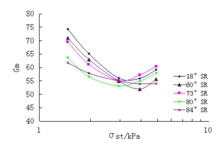
**Fig. 4.** The  $G_m$ - $\sigma_{st}$  curves of foam buffer materials prepared with micronized fibers of different beating degrees
