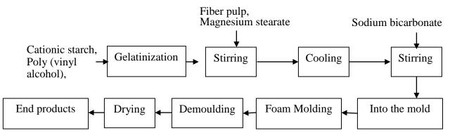
Fig. 1. The flow chart of the preparation of foam buffer materials
