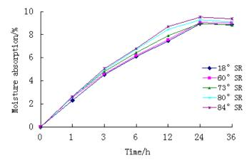
Fig. 2. Effects of the beating degree of micronized fibers on moisture absorption
