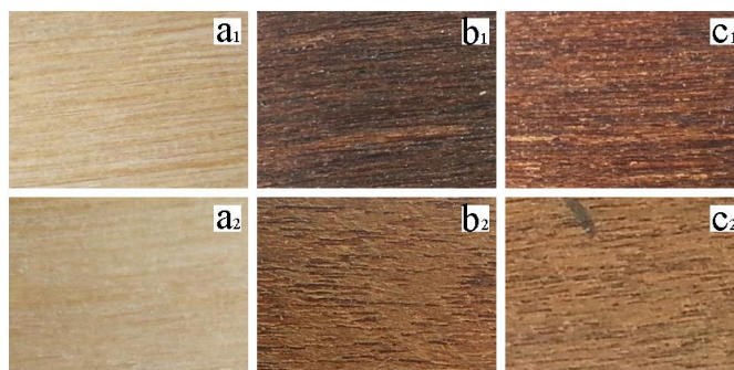
Fig. 1. Color of untreated and treated wood samples. Inside color: (a 1 ) untreated wood; (b 1 ) FA-treated wood; and (c 1 ) FA/SiO 2 -treated wood. Surface color: (a 2 ) untreated wood; (b 2 ) FA-treated wood; and (c 2 ) FA/SiO 2 -treated wood
