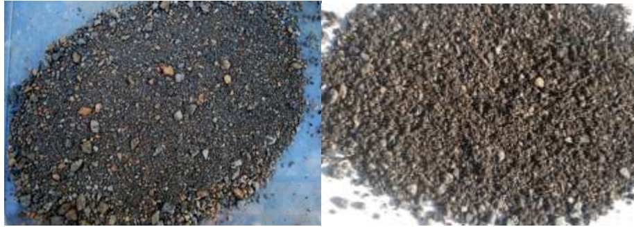
Fig. 2. Left: calcined clay; Right: calcined clay with red oak biochar added
