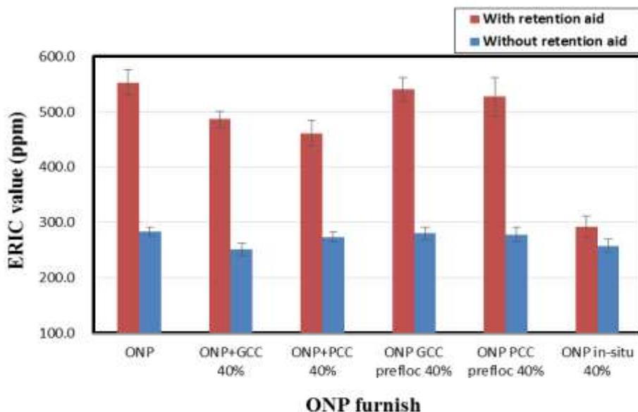
**Fig. 5.** ERIC values of handsheets from ONP furnishes with 40%  $\text{CaCO}_3$  ash content and with and without 0.1% PAM addition
