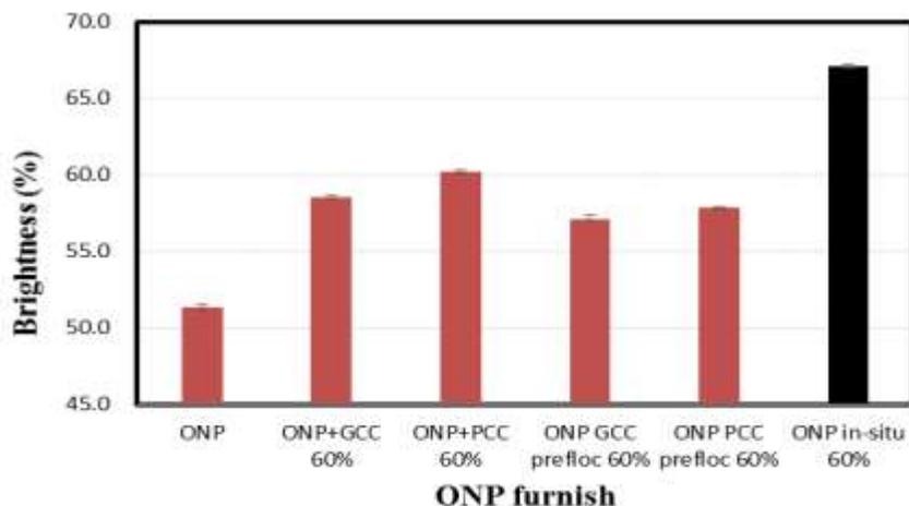
**Fig. 4.** ISO brightness of handsheets from ONP furnishes with 60% CaCO<sub>3</sub> ash content and 0.1% PAM addition
