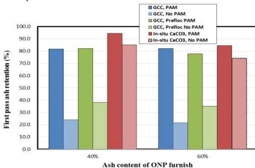
Fig. 1. First-pass retention of GCC and *in-situ* CaCO<sub>3</sub> in ONP
