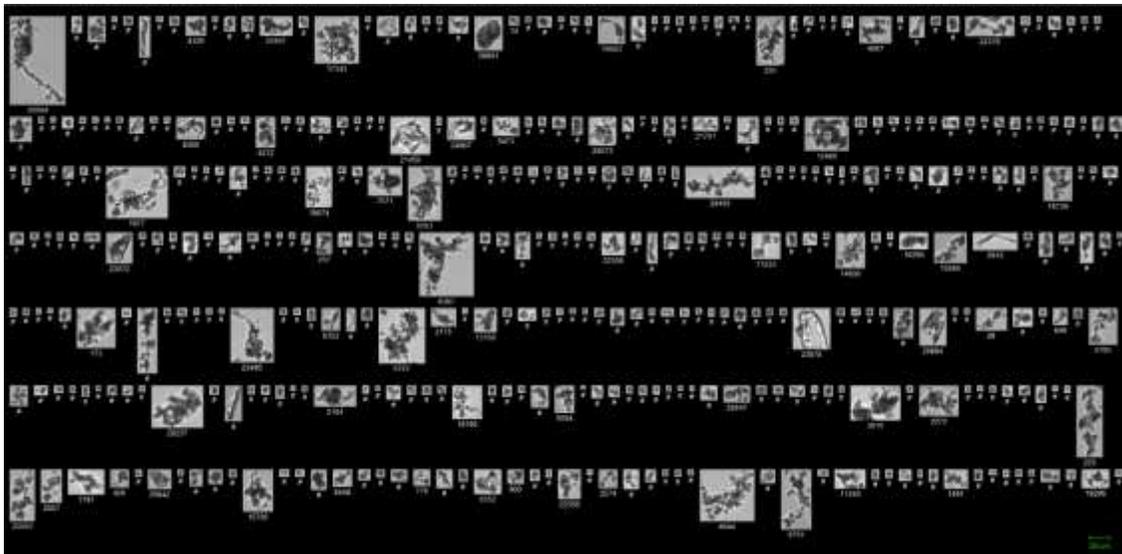
**Fig. 14.** Optical image of the fine fraction at *in-situ* CaCO<sub>3</sub> 60% (FlowCAM® dynamic imaging particle analyzer)
