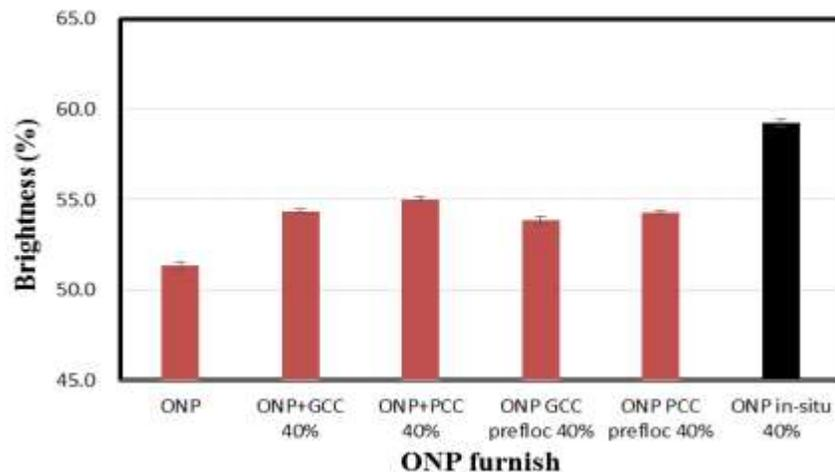
**Fig. 3.** ISO brightness of handsheets from ONP furnishes with 40% CaCO<sub>3</sub> ash content and 0.1% PAM addition
