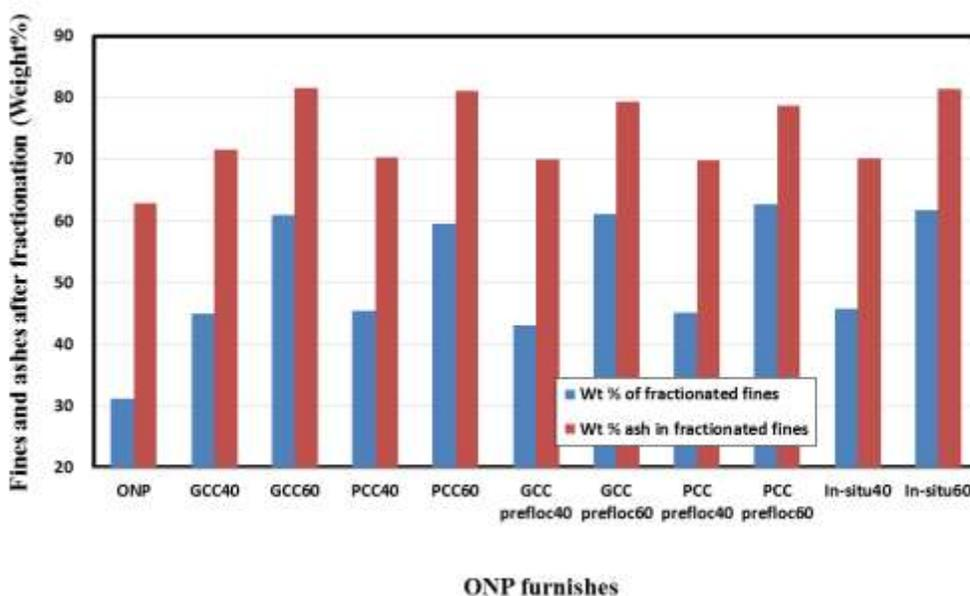
Fig. 9. The weight% and ash contents of fractionated fines in ONP
