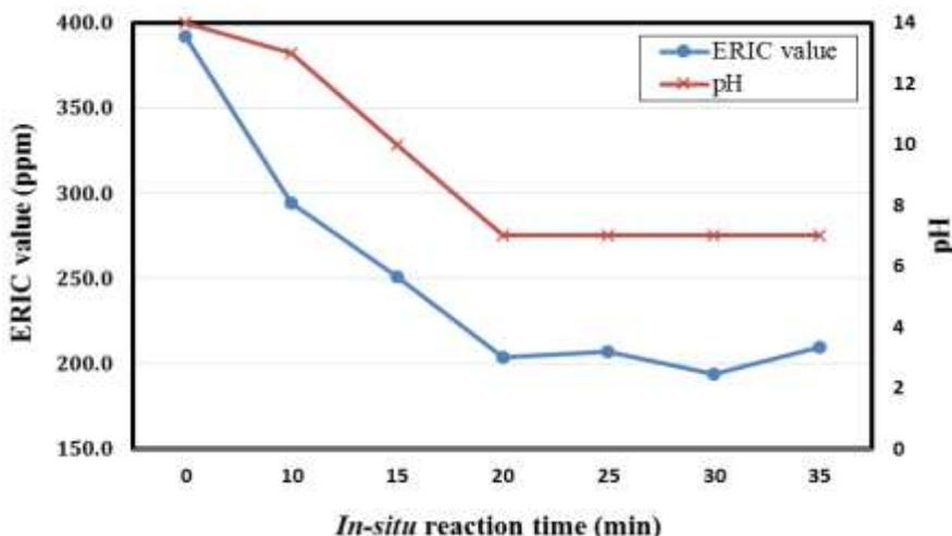
Fig. 8. ERIC value and furnish pH as a function of reaction time of *in-situ* CaCO<sub>3</sub> formation
