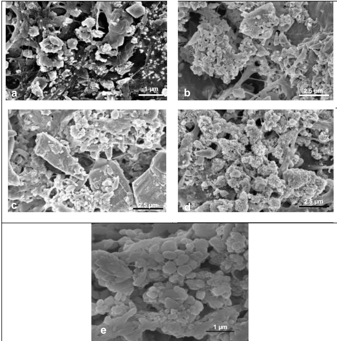
**Fig. 15.** SEM micrographs of ONP fractionated fines. (a) No CaCO<sub>3</sub> added, (b) PCC added, (c) pre-flocculated PCC, (d) *in-situ* CaCO<sub>3</sub>, and (e) magnified image of the *in-situ* CaCO<sub>3</sub>
