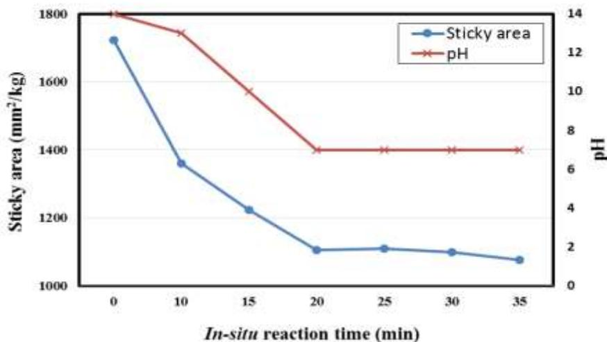
**Fig. 7.** The macro sticky area and furnish pH as a function of reaction time of *in-situ*  $\text{CaCO}_3$  formation
