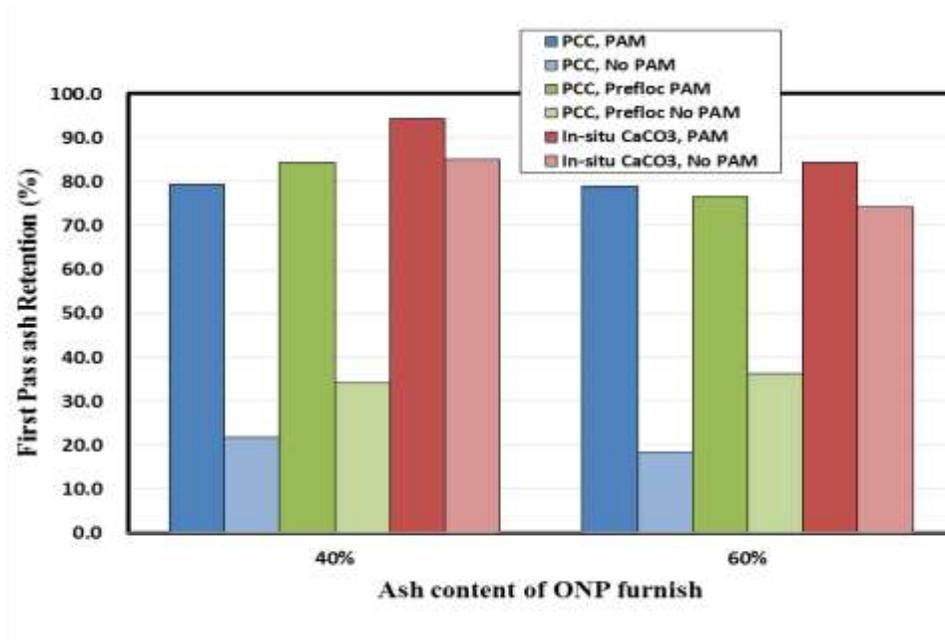
**Fig. 2.** First-pass retention of PCC and *in-situ* CaCO<sub>3</sub> in ONP
