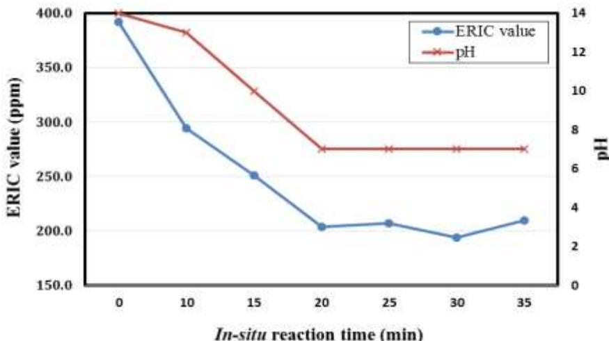
Fig. 8. ERIC value and furnish pH as a function of reaction time of *in-situ* CaCO<sub>3</sub> formation
