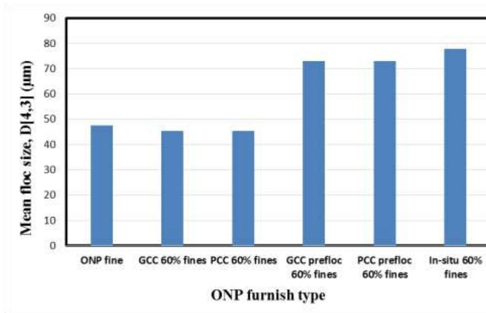
Fig. 10. Size of fractionated fines measured by FlowCAM® dynamic imaging particle analyzer
