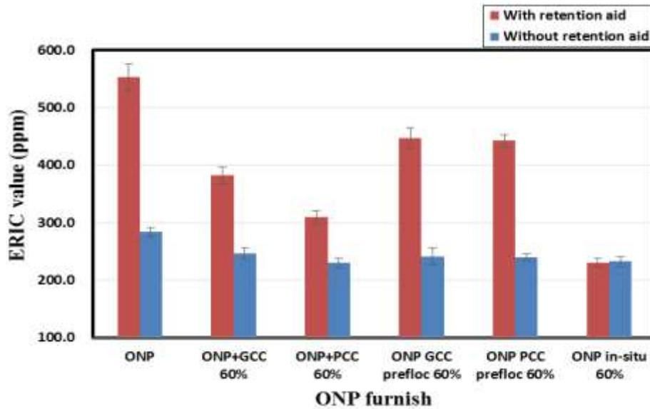
**Fig. 6.** ERIC values of handsheets from ONP furnishes with 40%  $\text{CaCO}_3$  ash content and with and without 0.1% PAM addition
