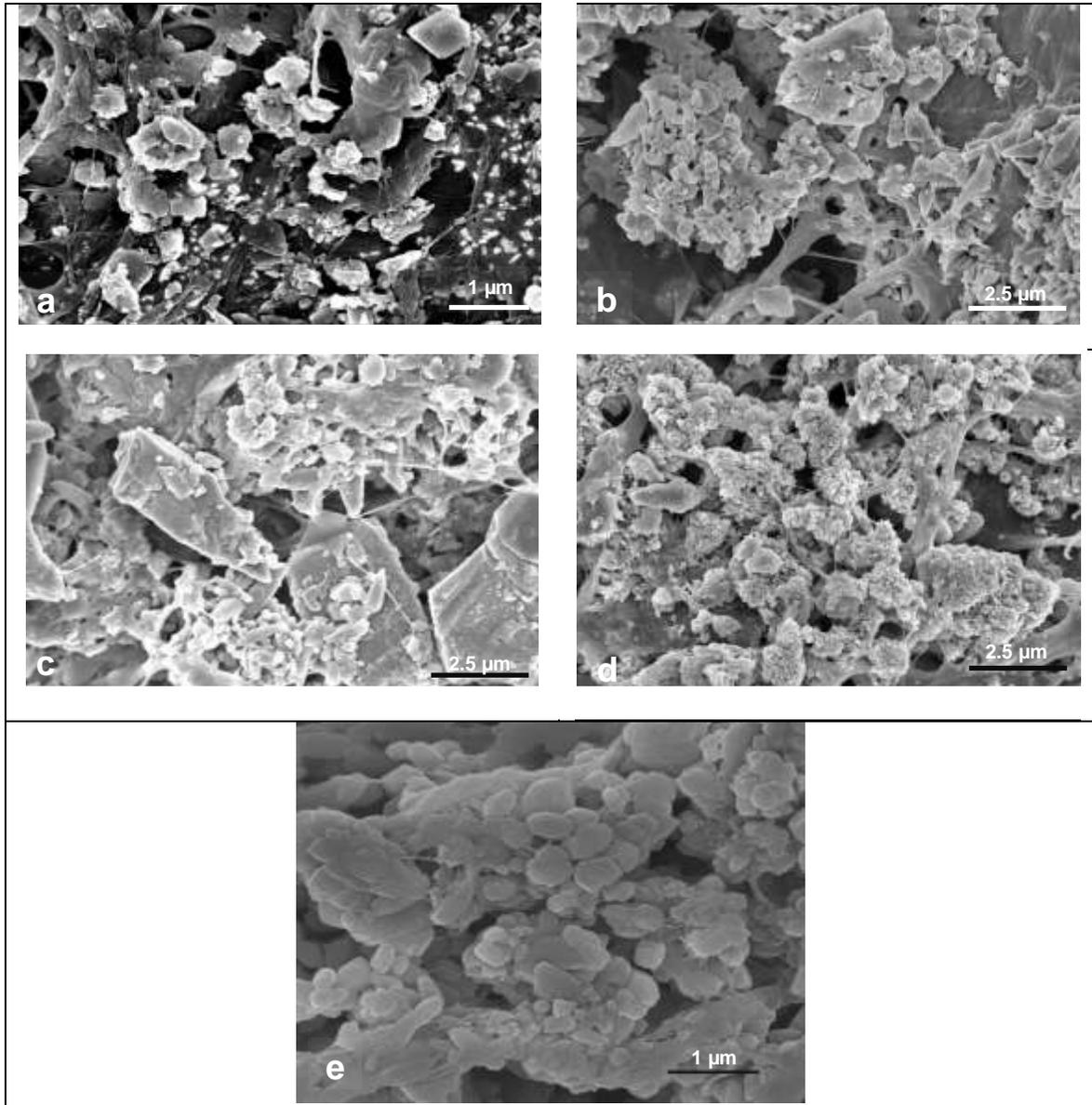
**Fig. 15.** SEM micrographs of ONP fractionated fines. (a) No  $\text{CaCO}_3$  added, (b) PCC added, (c) pre-flocculated PCC, (d) *in-situ*  $\text{CaCO}_3$ , and (e) magnified image of the *in-situ*  $\text{CaCO}_3$
