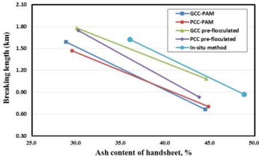
Fig. 11. Breaking lengths of handsheets from ONP furnishes with addition of  $\text{CaCO}_3$
