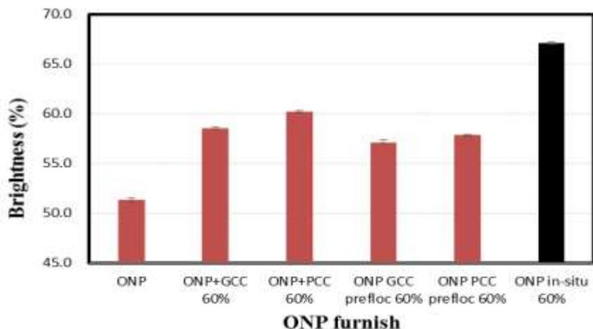
**Fig. 4.** ISO brightness of handsheets from ONP furnishes with 60%  $\text{CaCO}_3$  ash content and 0.1% PAM addition
