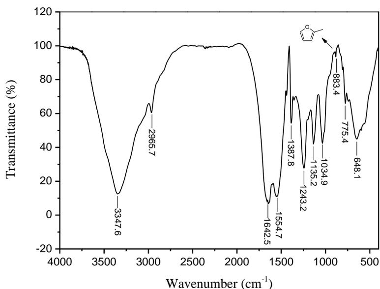
Fig. 3. The FTIR spectrum of the cured UFFR resin
