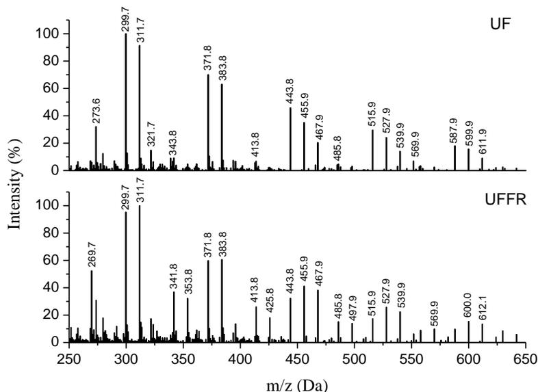
**Fig. 2.** Comparison of the MALDI-TOF spectra between UF resin and UFFR resin (250-650 Da)
