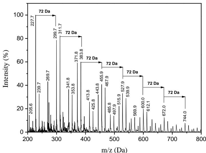
**Fig. 1.** The MALDI-TOF spectrum of the UFFR resin
