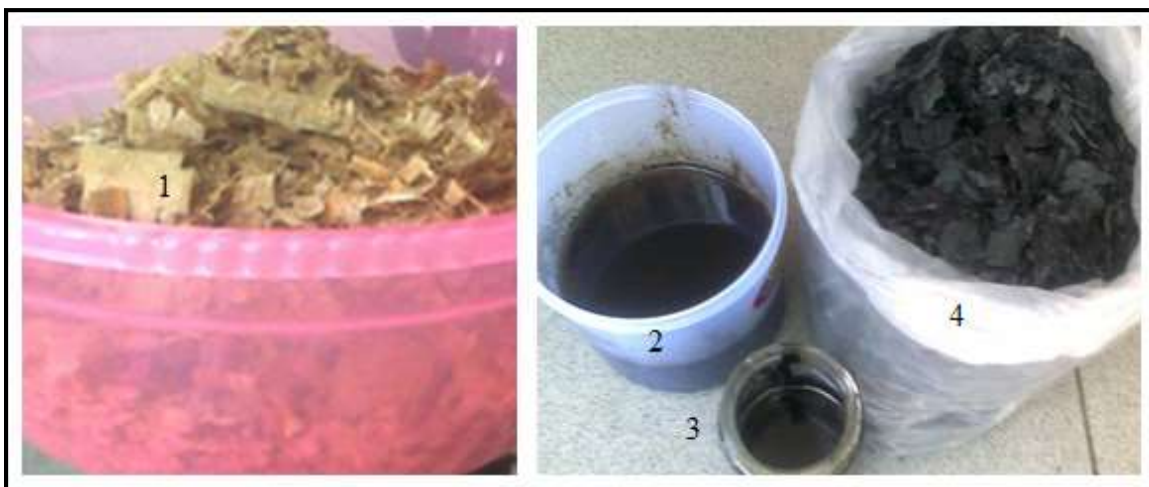
Fig. 4. (1) Chips of wood waste; (2) crude WV; (3) tar; and (4) char
