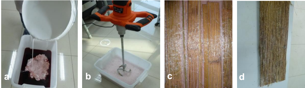
Fig. 1. Impregnation process for bamboo bundle fiber with PF/PVAC resin. (a) Glue preparation, (b) blending, (c) dipping, and (d) drying
