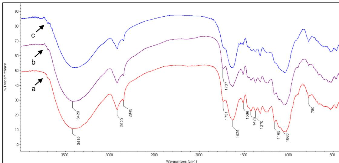
**Fig. 5.** FTIR spectra of (a) cassava residue, (b) Congo red-loaded cassava residue, and (c) Congo red-loaded cassava residue after *in vivo* decolorization
