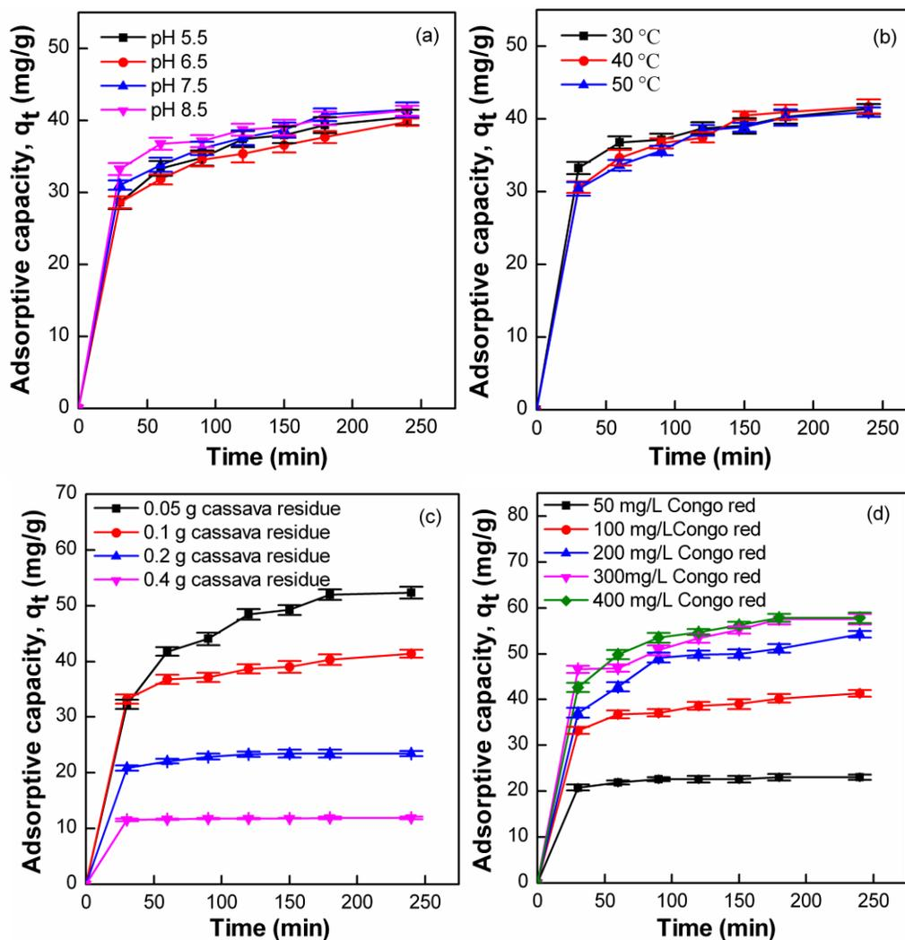
**Fig. 1.** Effect of: (a) pH at cassava residue dosages of 0.1 g, temperature of 30 °C, and Congo red concentration of 100 mg/L; (b) temperature at cassava residue dosages of 0.1 g, pH 8.5, and Congo red concentration of 100 mg/L; (c) cassava residue dosage at temperature of 30 °C, pH 8.5, and Congo red concentration of 100 mg/L; (d) Congo red concentration at temperature of 30 °C, pH 8.5, and cassava residue dosages of 0.1 g on the Congo red adsorptive capacity of cassava residue
