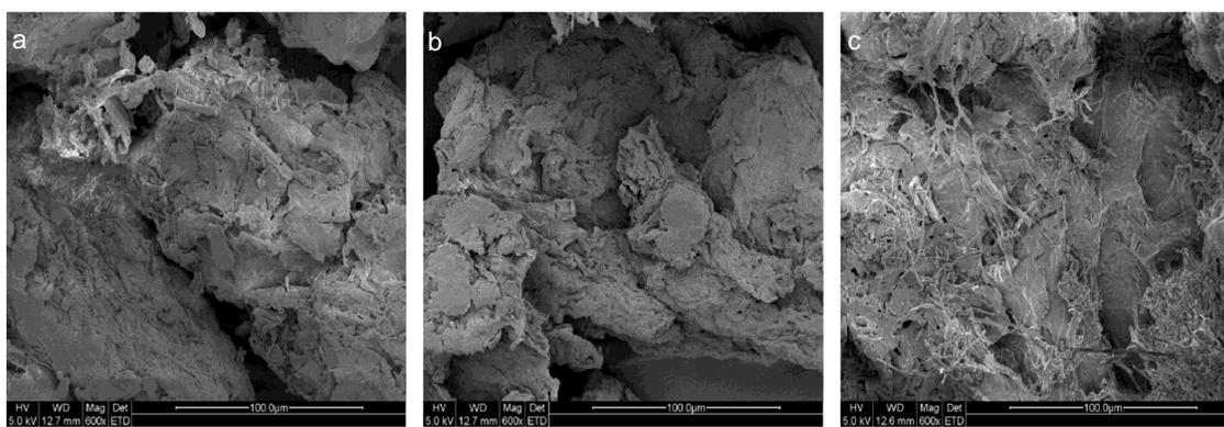
**Fig. 4.** SEM images (magnification  $\times 600$ ) of (a) cassava residue, (b) Congo red-loaded cassava residue, and (c) Congo red-loaded cassava residue after *in vivo* decolorization
