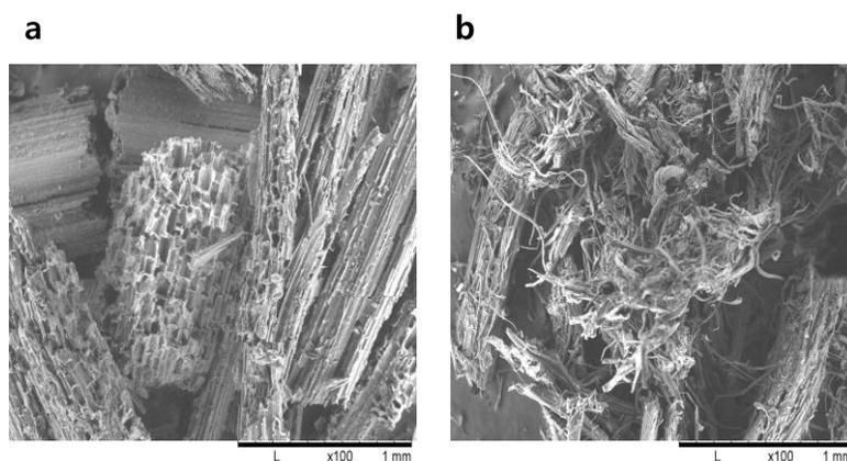
**Fig. 1.** Scanning electron microscopy (SEM) analysis. Micrographs from untreated (a) and treated (b) *Miscanthus* (x100)
