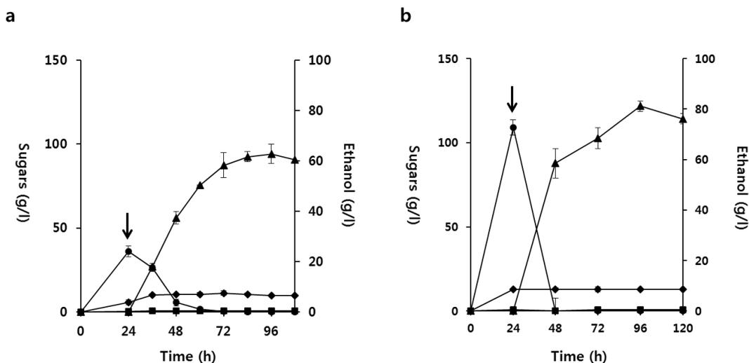
**Fig. 3.** Partial SSF kinetics with pretreated GU containing 12% glucan (a) and 16% glucan (b); ethanol (▲), glucose (●), xylose (◆), and arabinose (■). Fermentation was conducted in a 5-L reactor. Arrows indicate cell addition at 24 h. Bars represent standard deviation from three independent experiments
