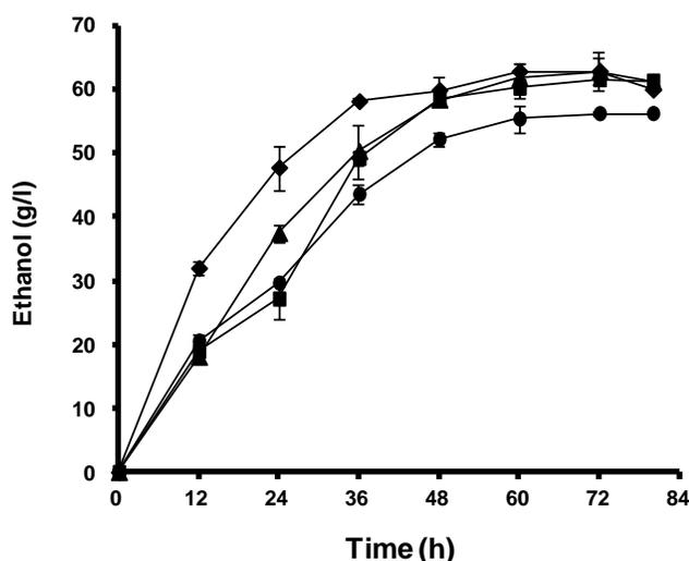
**Fig. 2.** Determination of additional nutrients for the SSF of pretreated GU. The fermentation mixture with YP and buffer (◆); with YP and without buffer (▲); without YP and with buffer (■); and without YP and buffer (●). Bars represent standard deviation from two independent experiments
