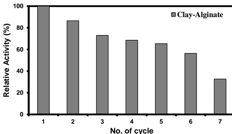
Fig. 6. Reusability of alginate-clay beads in tapioca slurry hydrolysis process
