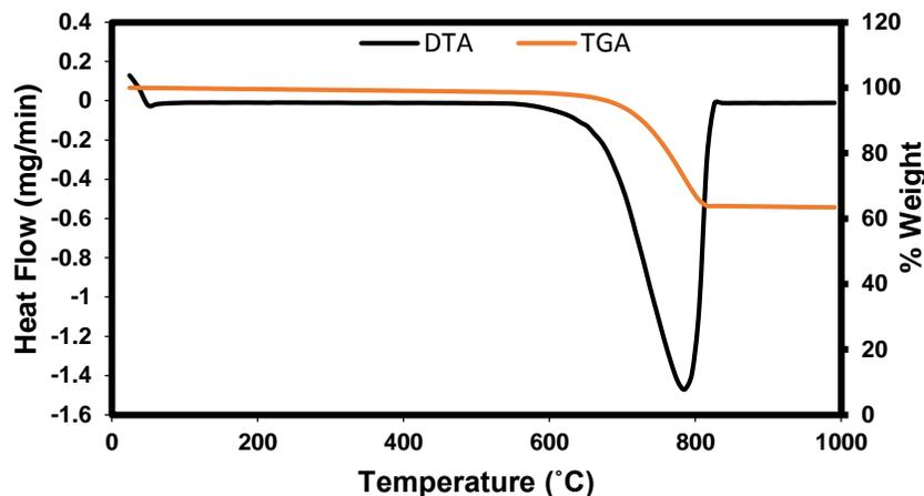
**Fig. 3.** Differential thermal and thermogravimetric analysis of waste clay sample
