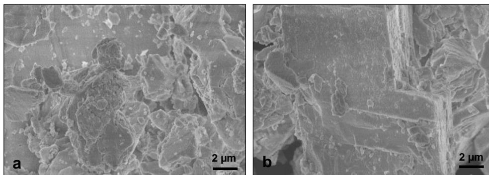
**Fig. 4.** FESEM micrograph of waste clay at 5000x magnification at two different spots
