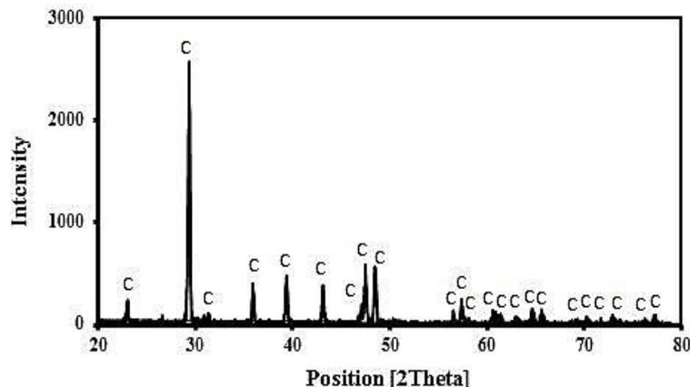
Fig. 1. X-ray diffraction (XRD) pattern of waste clay. C=calcite
