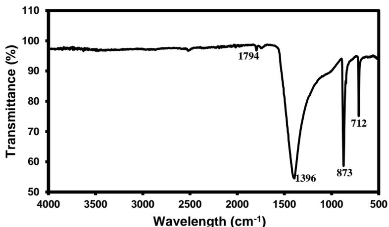
Fig. 2. FTIR spectra of waste clay
