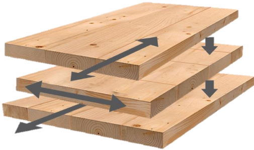
Fig. 1. Schematic of CLT layer configuration
