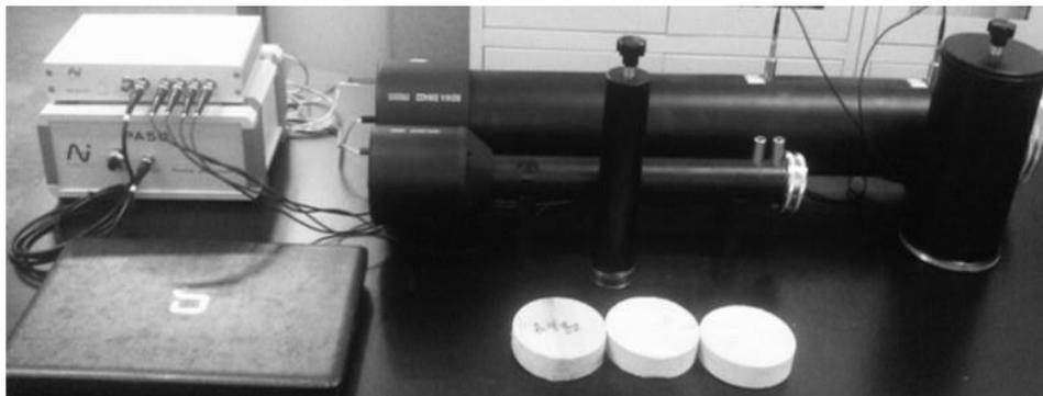
**Fig. 1.** Impedance tubes and samples
