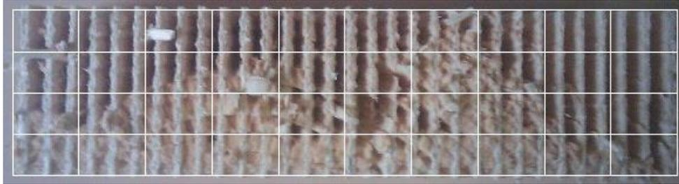
**Fig. 4.** Principle of visual evaluation of fracture area
