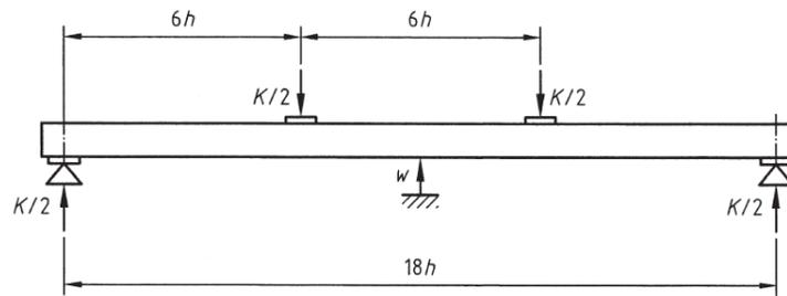
**Fig. 3.** Test arrangement for measuring global modulus of elasticity and bending strength
