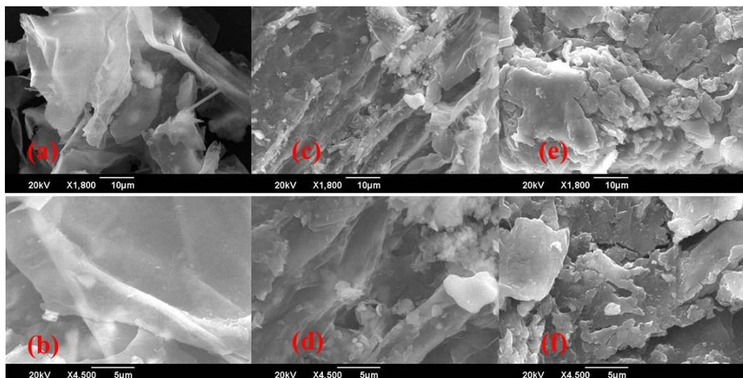
**Fig. 1.** SEM images of water hyacinth. (a) raw biomass of water hyacinth at 1800 $\times$ , (b) raw biomass of water hyacinth at 4500 $\times$ , (c) pretreated water hyacinth with microwave-assisted alkaline at 1800 $\times$ , (d) pretreated water hyacinth with microwave-assisted alkaline at 4500 $\times$ , (e) pretreated water hyacinth with microwave-assisted acid at 1800 $\times$ , (f) pretreated water hyacinth with microwave-assisted acid at 4500 $\times$ .
