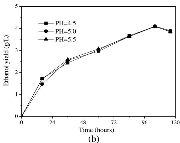
**Fig. 7.** Effects of pH on the ethanol yield of water hyacinth pretreated with microwave and acid under high pressure through a simultaneous saccharification and fermentation process with yeasts: (a) *S. cerevisiae* and (b) *P. stipitis*
