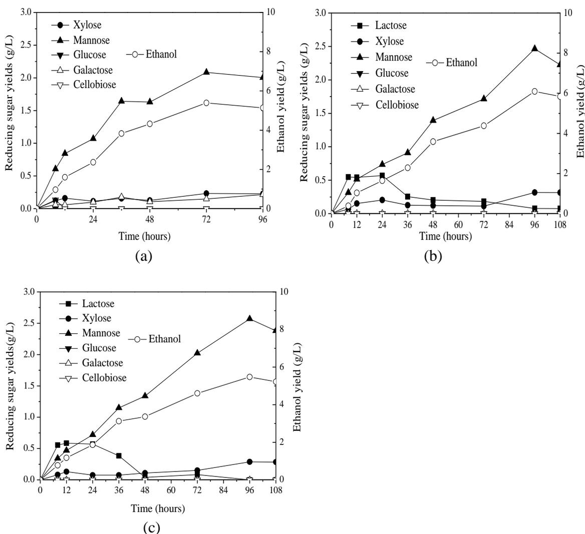
**Fig. 5.** Ethanol and reducing sugar yield of water hyacinth pretreated with microwave and lightwave-assisted alkali through a simultaneous saccharification and fermentation process with yeasts: (a) *S. cerevisiae*, (b) *P. tannophilus*, and (c) mixed *S. cerevisiae* and *P. tannophilus*. The ratio of microwave power to lightwave power was 3:7.
