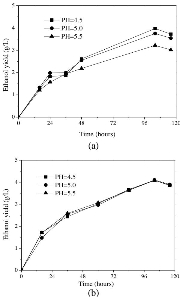
**Fig. 7.** Effects of pH on the ethanol yield of water hyacinth pretreated with microwave and acid under high pressure through a simultaneous saccharification and fermentation process with yeasts: (a) *S. cerevisiae* and (b) *P. stipitis*
