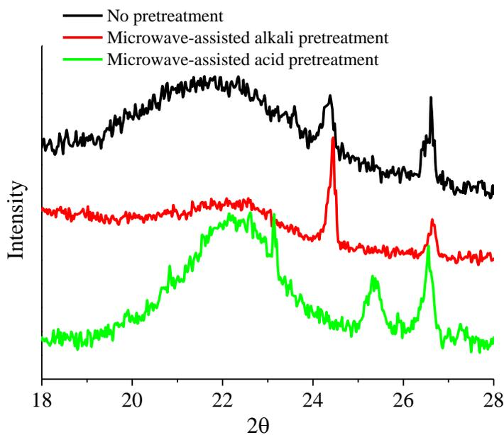
**Fig. 3.** XRD patterns of pretreated water hyacinth with microwave-assisted alkali or acid
