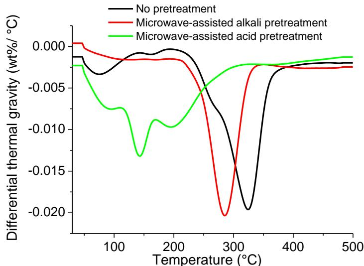
**Fig. 4.** TGA analysis of pretreated water hyacinth with microwave-assisted alkali or acid
