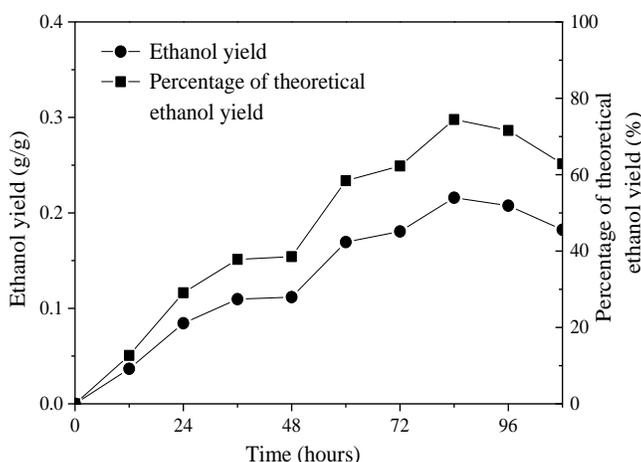
**Fig. 8.** Ethanol yield of water hyacinth pretreated with microwave and acid under high pressure through a simultaneous saccharification and fermentation process with acclimatized yeasts
