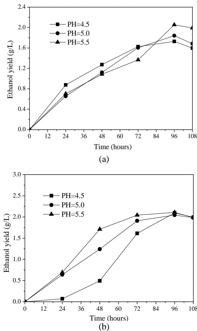
**Fig. 6.** Effects of pH on the ethanol yield of water hyacinth pretreated with microwave and alkali under high pressure through a simultaneous saccharification and fermentation process with yeasts: (a) *S. cerevisiae* and (b) *P. stipitis*
