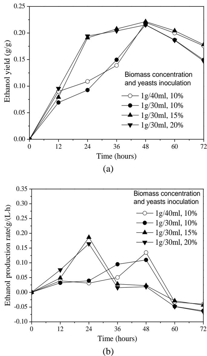
**Fig. 9.** Effects of the feedstock biomass concentration and acclimatized yeast inoculation amount on ethanol production yield (a) and rate (b) of water hyacinth pretreated with microwave and acid under high pressure
