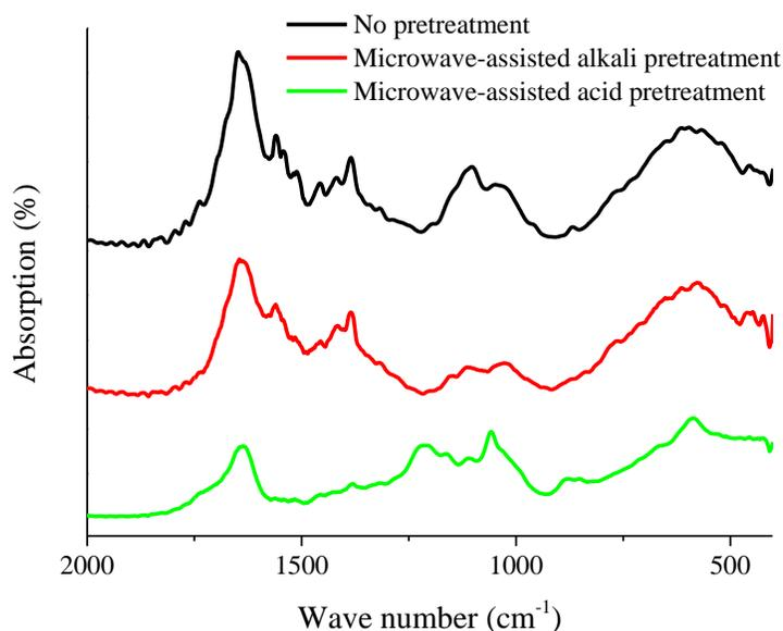
**Fig. 2.** FTIR spectra of pretreated water hyacinth with microwave-assisted alkali or acid
