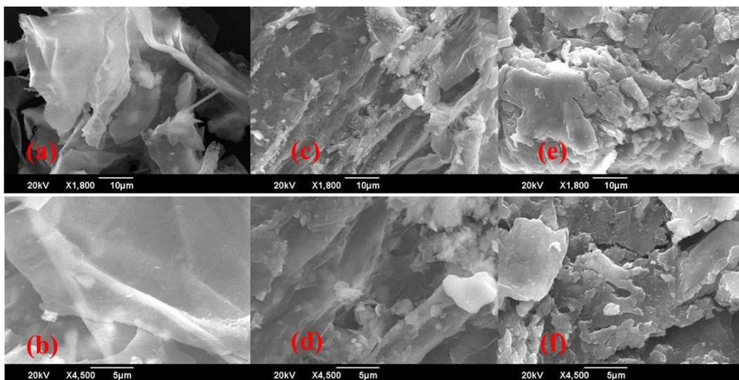
**Fig. 1.** SEM images of water hyacinth. (a) raw biomass of water hyacinth at 1800 $\times$ , (b) raw biomass of water hyacinth at 4500 $\times$ , (c) pretreated water hyacinth with microwave-assisted alkaline at 1800 $\times$ , (d) pretreated water hyacinth with microwave-assisted alkaline at 4500 $\times$ , (e) pretreated water hyacinth with microwave-assisted acid at 1800 $\times$ , (f) pretreated water hyacinth with microwave-assisted acid at 4500 $\times$ .
