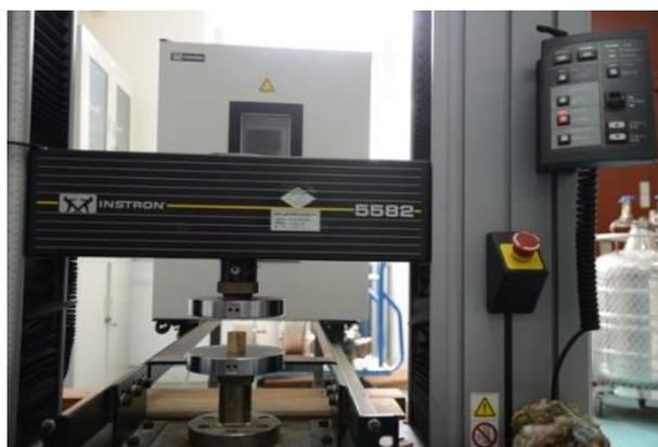
Fig. 4. Test set-up of compressive strength
