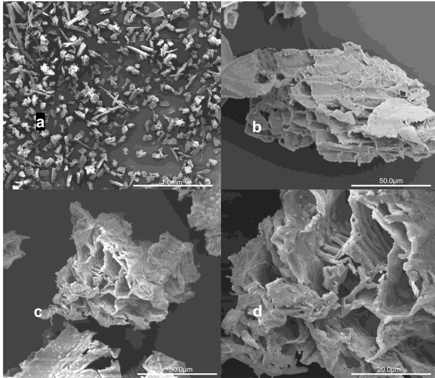
**Fig. 5.** SEM images of particles obtained through grinding and fractionation
