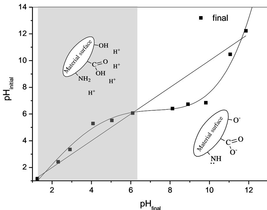
**Fig. 4.** Point of zero charge (pHpzc) determination for surface particles of corn leaf powder
