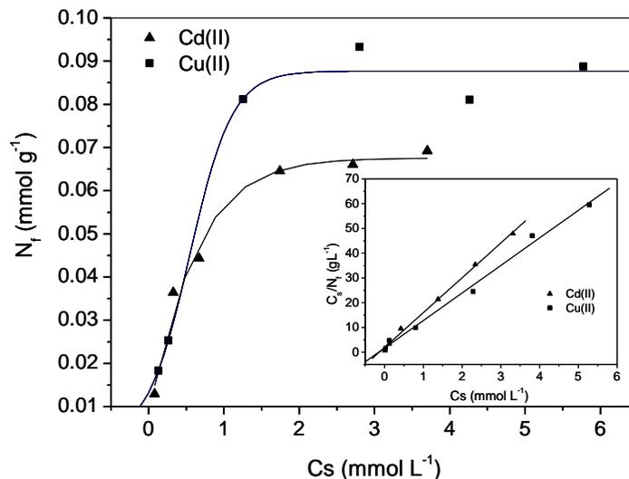
**Fig. 8.** Adsorption isotherms for Cu(II) and Cd(II) in aqueous solution at room temperature (28 °C) and linear shape of adsorption isotherms of Cu(II) and Cd(II) (inset)
