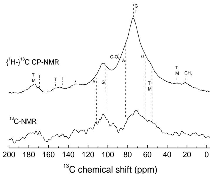
**Fig. 2.**  $^{13}\text{C}$  NMR spectra obtained through  $\{^1\text{H}\}$ - $^{13}\text{C}$  cross-polarization technique (upper trace) and with direct polarization of  $^{13}\text{C}$  (lower trace). Code for resonance identification: T= thiamine, M= methionine, G= glucoside, A= apiosyl.
