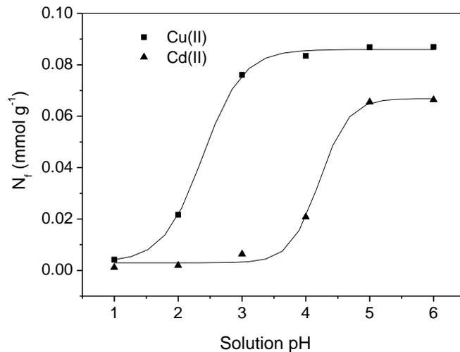
**Fig. 7.** Effect of solution pH on adsorption of Cu(II) and Cd(II) in aqueous medium
