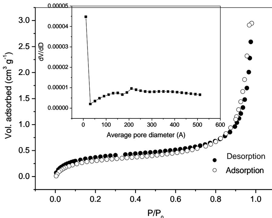
**Fig. 6.** Nitrogen adsorption and desorption isotherms and distribution of pore diameter (inserted figure)
