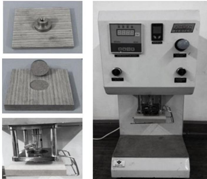
Fig. 1. Pull-off test instrument and specimens used in the study
