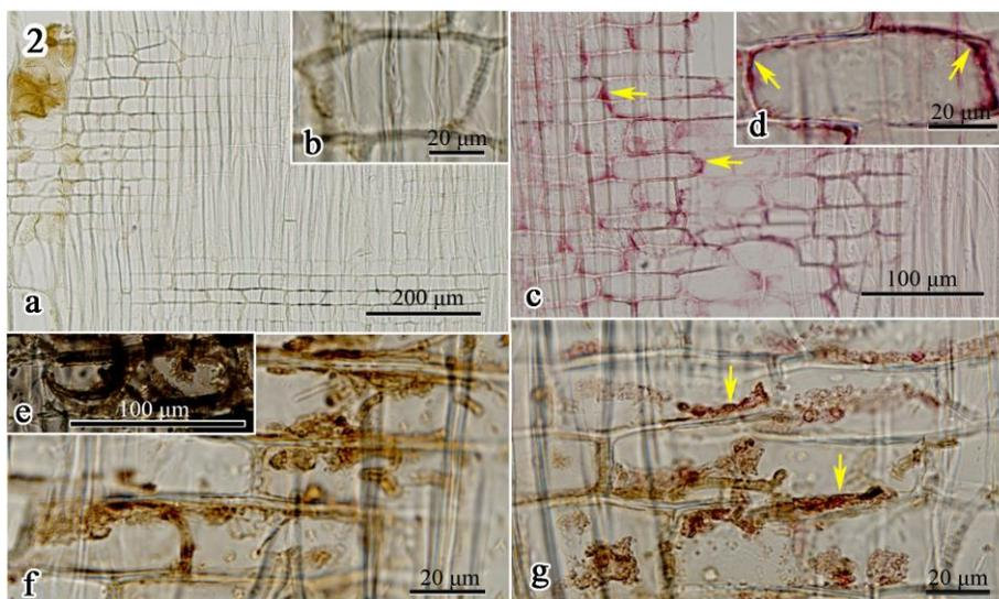
**Fig. 2.** Radial sections of *A. sinensis*. a, b and f: Control samples. c, d, e and g: Samples stained with aceto-carminé. a: Rays of sapwood. b: Magnification of a. c: Rays of sapwood. d: Magnification of c. e: Rays of heartwood of air-dried wood. f and g: Rays of heartwood of fresh wood. Parts indicated by arrows are nuclear chromatin in figure c, d and g
