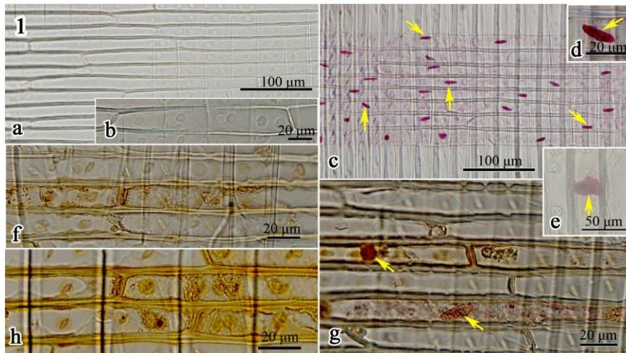
**Fig. 1.** Radial sections of *C. lanceolata*. a, b and h: Control samples. c, d, e, f and g: Samples stained with aceto-carminé. a: Rays of sapwood of fresh wood. b: Magnification of a. c: Rays of sapwood of fresh wood. d: Magnification of d. e: Axial parenchyma cells of fresh wood. f and g: Rays of heartwood of fresh wood. h: Rays of heart of air-dried wood. Parts indicated by arrows are nuclei in figure c, d, e, and g
