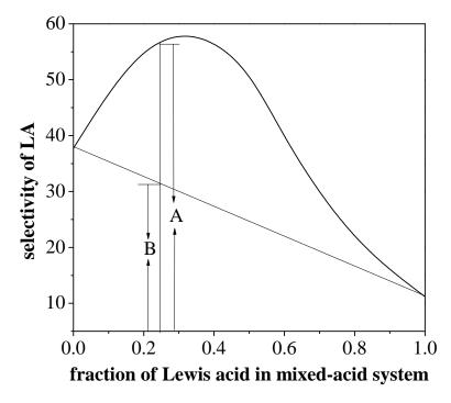
Fig. 1. The definition of A and B related to synergy factor in mixed-acid system
