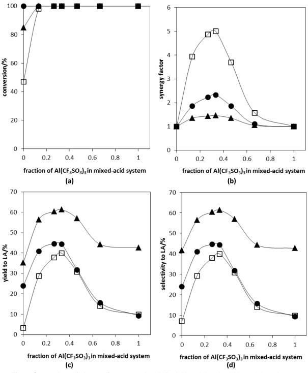
**Fig. 3.** Conversions of glucose, fructose, and 5-HMF, yields to LA, selectivities to LA, and synergy factors in hydrothermal decomposition. Reaction condition: concentration of glucose, fructose, or 5-HMF = 0.0556 mol/L, concentration of Al(CF<sub>3</sub>SO<sub>3</sub>)<sub>3</sub> + H<sub>2</sub>C<sub>2</sub>O<sub>4</sub> = 0.015mol/L, temperature = 180 °C, reaction time = 5 h.  $\Box$ -glucose,  $\bullet$ -fructose,  $\blacktriangle$ -5-HMF
