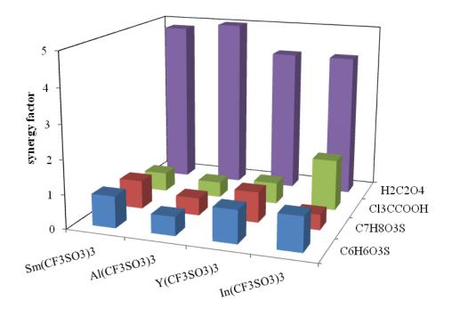
**Fig. 2.** Synergy factors for glucose decomposition with organic Brønsted acid and Lewis acid at 180 °C for 5 h. Concentration in mixed-acid system: Brønsted acid = 0.01 mol/L, Lewis acid = 0.005 mol/L, glucose = 0.0556 mol /L.
