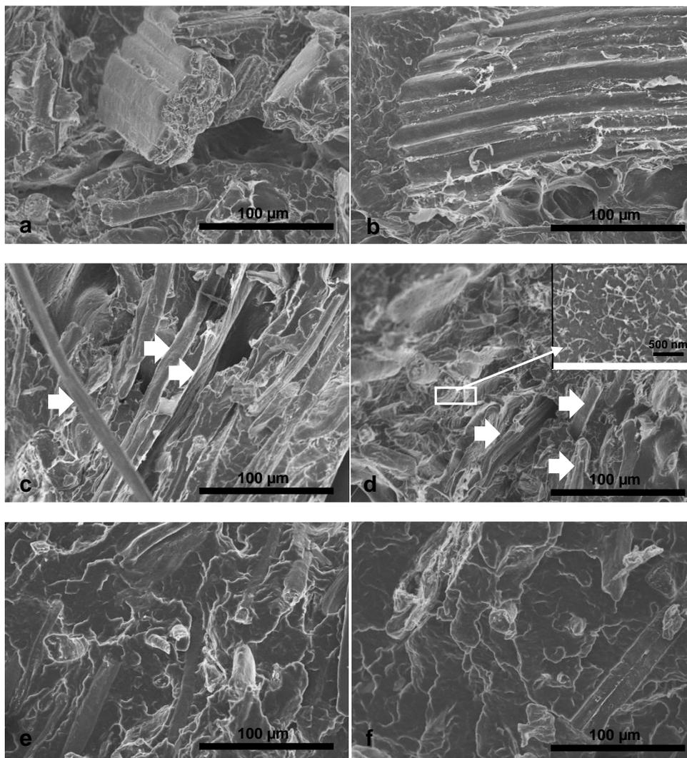
**Fig. 4.** Morphology of fracture surfaces produced by tensile testing composites of: (a) PP/BF (50/50); (b) PP/BF (50/50) with 5 phr MAPP; (c) PP/HCW-treated BF (50/50); (d) PP/HCW-treated BF (50/50) with 5% MAPP; (e) PP/HCW-treated BF (70/30) with 5 phr MAPP; and (f) PP/HCW-treated BF (90/10) with 5 phr MAPP. Note that both (e) and (f) are samples that were prepared by re-compounding from a 50/50 master batch composite
