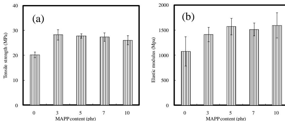
**Fig. 3.** Effect of MAPP content on the tensile strength (a) and elastic modulus (b) of a PP/HCW-treated (170 °C) BF (70/30) composite prepared from a master batch compound (PP/BF = 50/50). Data provided as the mean  $\pm$  standard deviation
