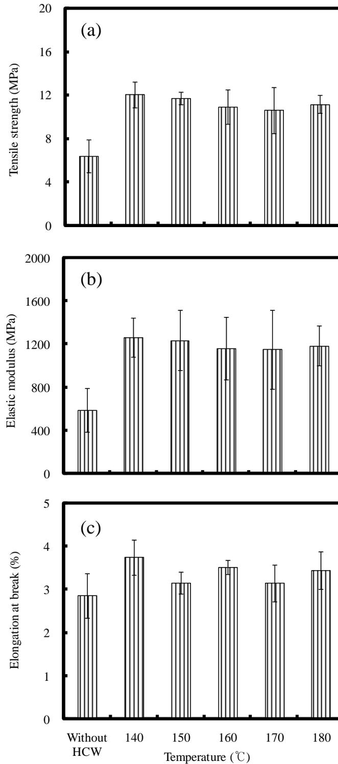
**Fig. 1.** Effect of varying the temperature at which BF is treated by HCW on the tensile strength (a), elastic modulus (b), and elongation at break (c) of a PP/BF (50/50) composite. Data provided as the mean  $\pm$  standard deviation
