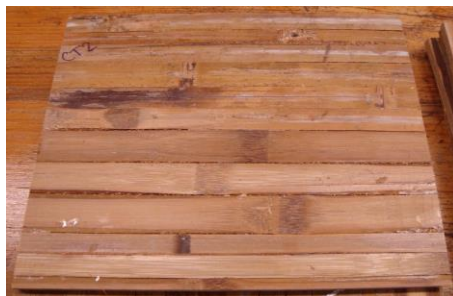
Fig. 1. Particleboard manufactured with bamboo waste and reinforced with bamboo laminas
