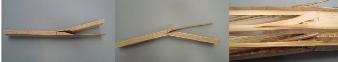
Fig. 2. Types of ruptures after the static bending test
