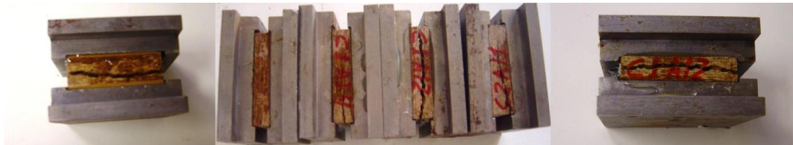
Fig. 3. Boards without reinforcement after internal adhesion test
