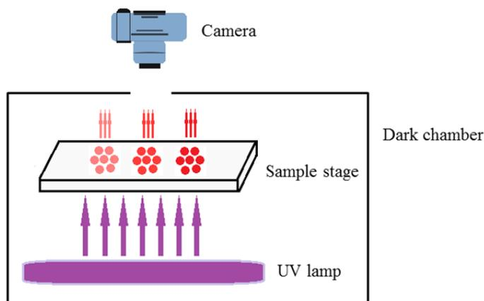
**Fig. 1.** Schematic diagram of the fluorescence imaging system assembled in-house.
