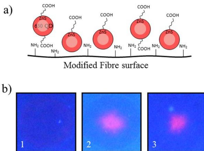
**Fig. 2.** a) Possible schemes of the QDs captured by modified cellulose paper' b) Fluorescence images of QDs on cellulose paper (1) without modification, (2) with APTMS-modification, (3) with chitosan modification
