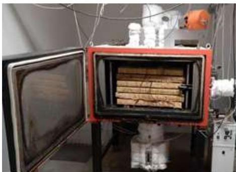
Fig. 2. Laboratory thermal furnace S250/03
