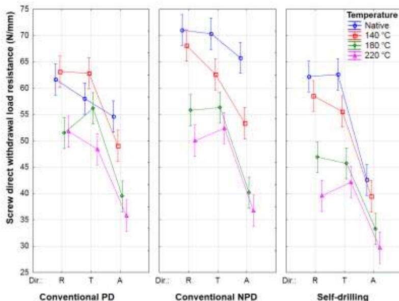
**Fig. 10.** A 95% confidence interval shows the influence of temperature, screw type and anatomical direction on screw direct withdrawal load resistance
