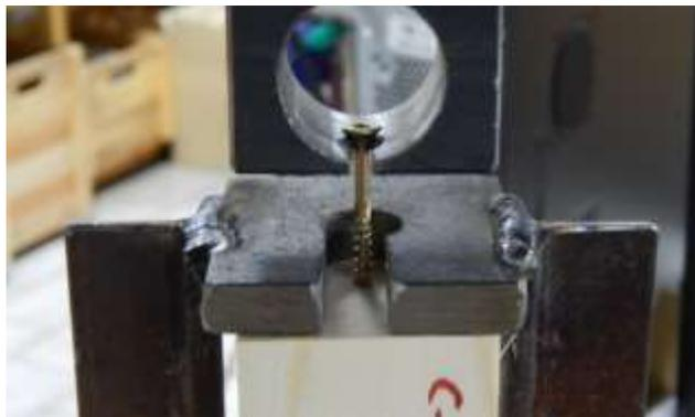
**Fig. 6.** Placement of the sample in extraction jig
