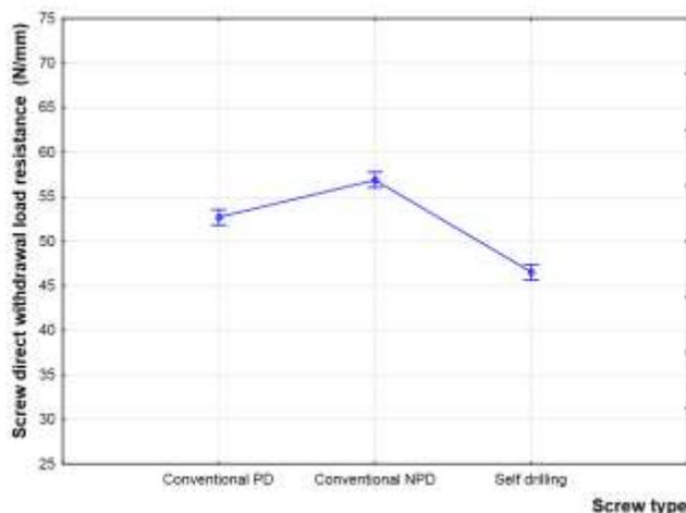
**Fig. 8.** A 95% confidence interval shows the influence of screw type on screw direct withdrawal load resistance
