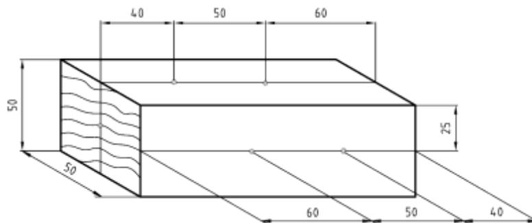
**Fig. 4.** Marking of test samples for insertion of screws
