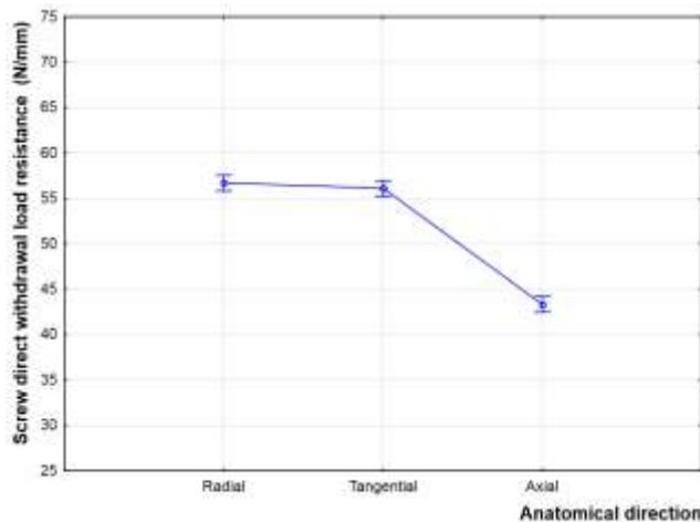
**Fig. 9.** A 95% confidence interval shows the influence of anatomical direction on screw direct withdrawal load resistance
