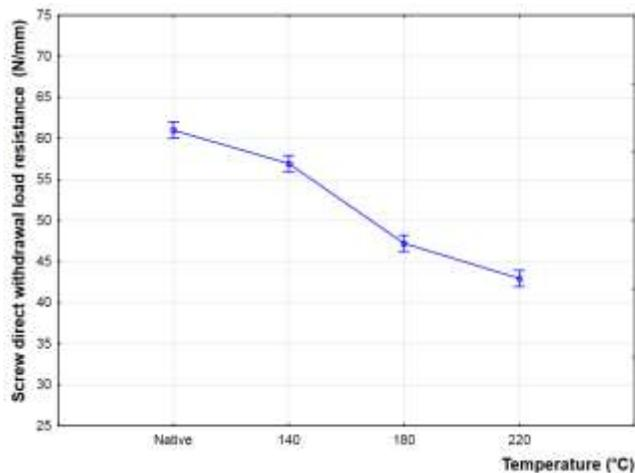
**Fig. 7.** A 95% confidence interval shows the influence of temperature on screw direct withdrawal load resistance
