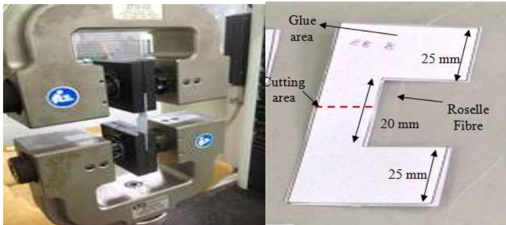
Fig. 2. Tensile test for roselle fibre
