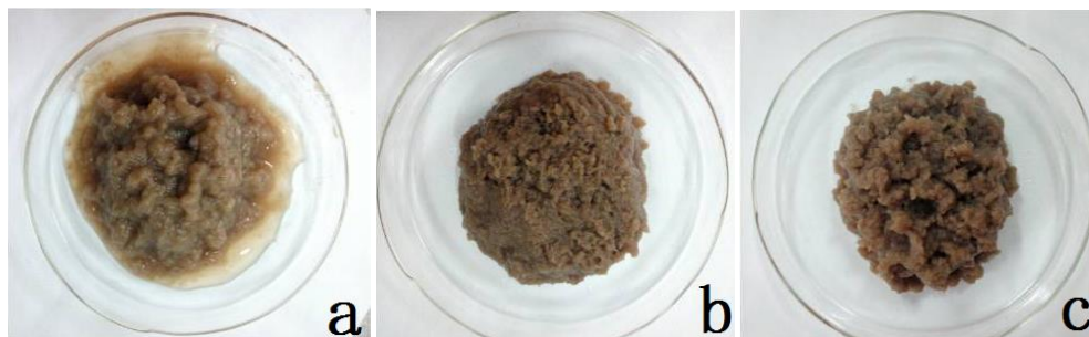
Fig. 2. Images of samples at various fiber concentrations (w/w%): (a) 5%, (b) 10%, and (c) 15%
