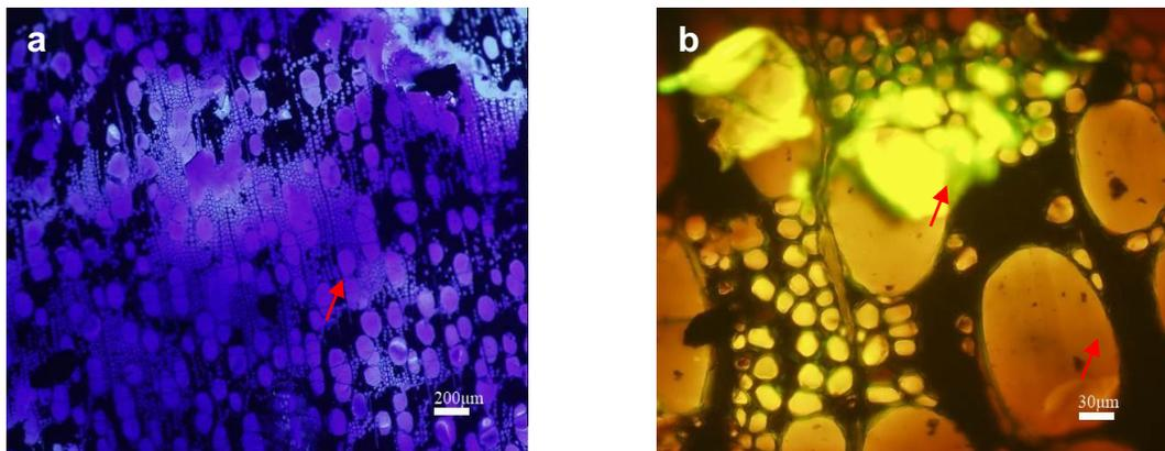
**Fig. 5.** Fluorescent micrographs of impregnated wood
