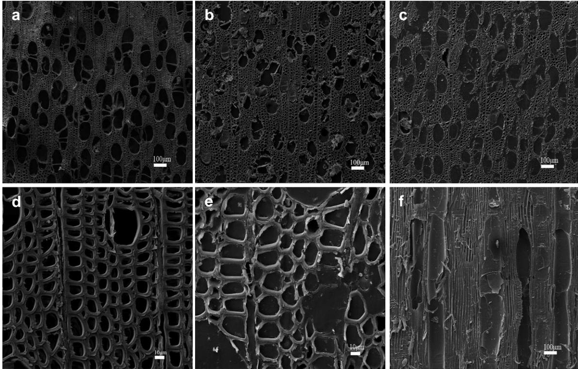
**Fig. 4.** SEM micrographs of control and RF resin impregnated wood. (a) Cross-section of control wood; (b) Cross-section of impregnated wood without microwave pretreatment; (c) Cross-section of impregnated wood with microwave pretreatment; (d) Cross-section of wood fiber in control wood; (e) Cross-section of wood fiber in impregnated wood; (f) Radial section of impregnated wood
