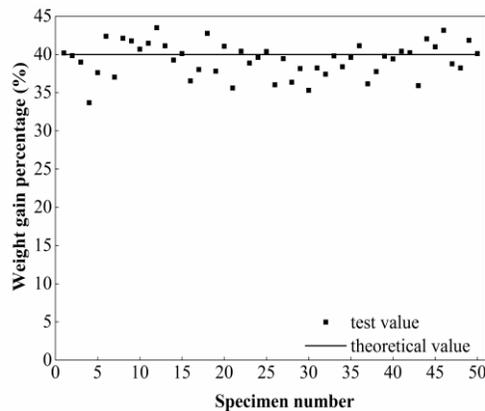
**Fig. 2.** Weight gain percentage for model validation
