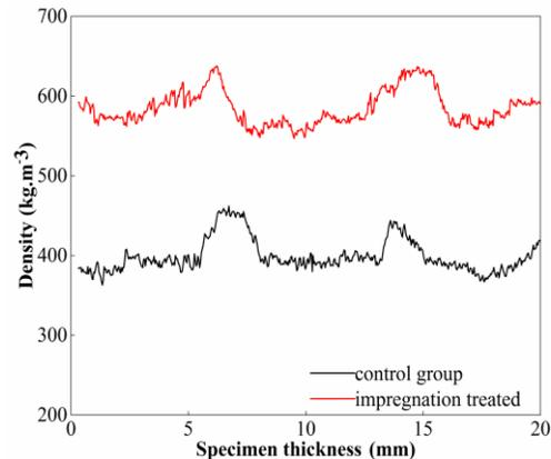
**Fig. 3.** Density distribution of untreated control and treated poplar by X-ray scanning
