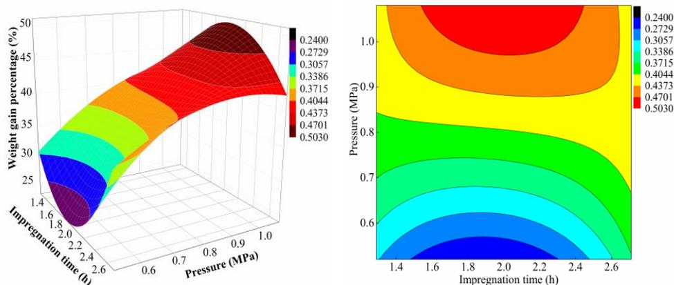
**Fig. 1.** Response surface and contour plots for the effect of interaction of two factors on weight gain percentage
