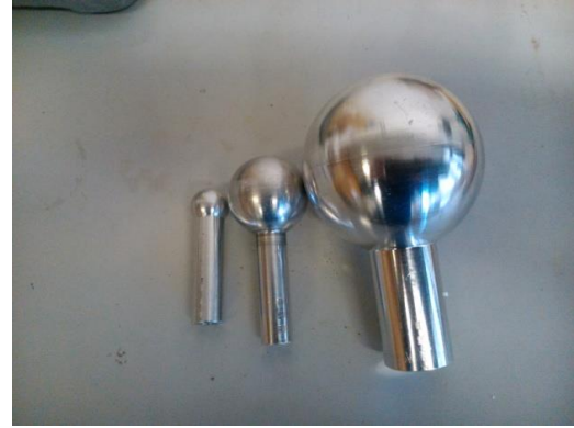
Fig. 4. Stamping tools of 3D-bending
