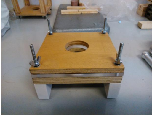
Fig. 3. 3D-bending testing jig
