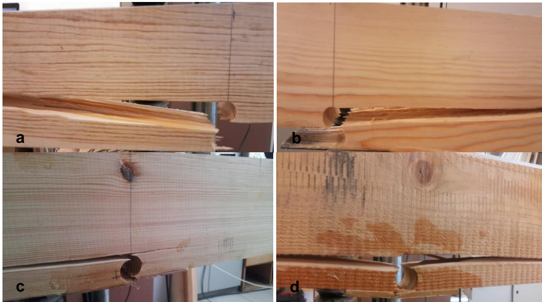
Fig. 12. Failure modes observed in (a) group A, (b) group B, (c) group C, and (d) group D
