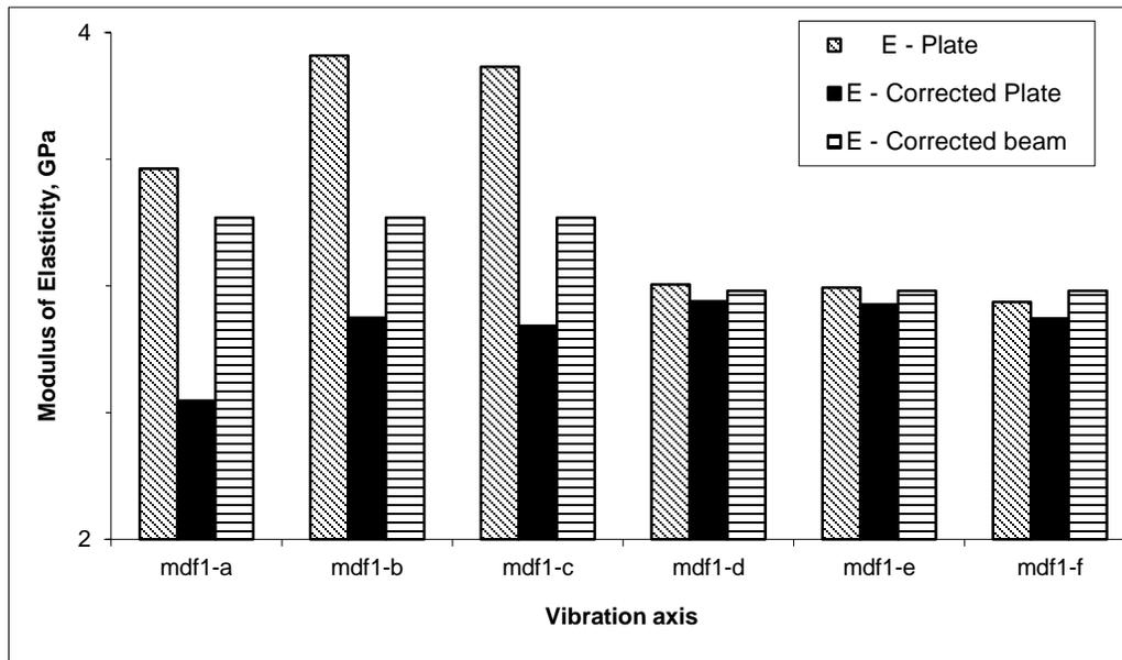
**Fig. 7.** Comparing vibration axes along the width and length. a, b, and c correspond to vibration along the width; d, e and f along the length. Brancheriau's correction coefficient was successfully homogenized the obtained results in whole plate vibration.
