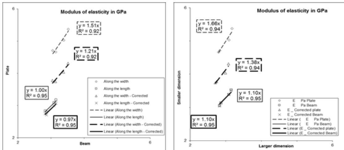
Fig. 6. Comparing the MDF2 plates with the prismatic beams (MDF4), with and without Brancheriau’s correction coefficient
