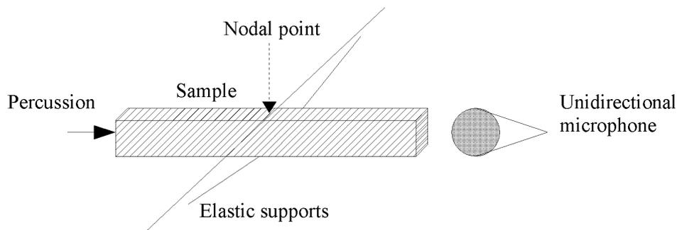
**Fig. 4.** Experimental setup, free-free bar in longitudinal vibration
