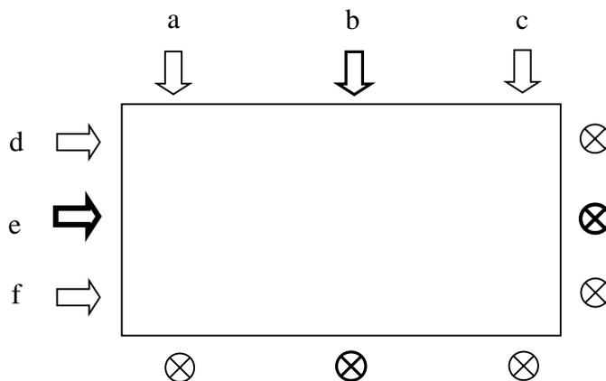
**Fig. 3.** Knocking and recording scenario on the whole plate in a, b, c, d, e and f directions; arrows are knocked perpendicular to thickness, parallel to the surface; the crossed-circles are the microphones. The smaller plates were knocked and recorded in shown in bold locations, in b and e directions, only.
