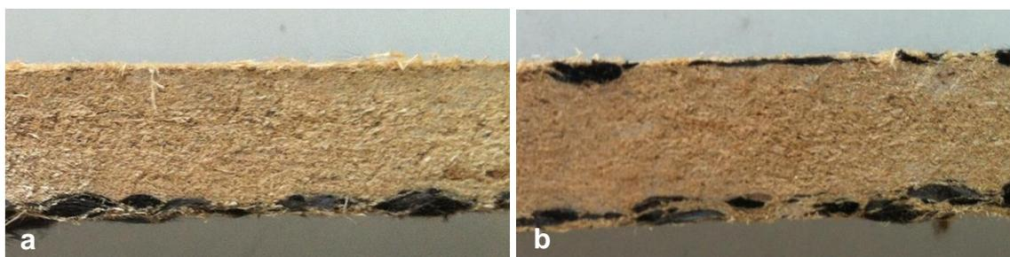
**Fig. 1.** Images of CFRWCs samples: (a) single-sided CFRWCs board; and (b) two-sided CFRWCs board
