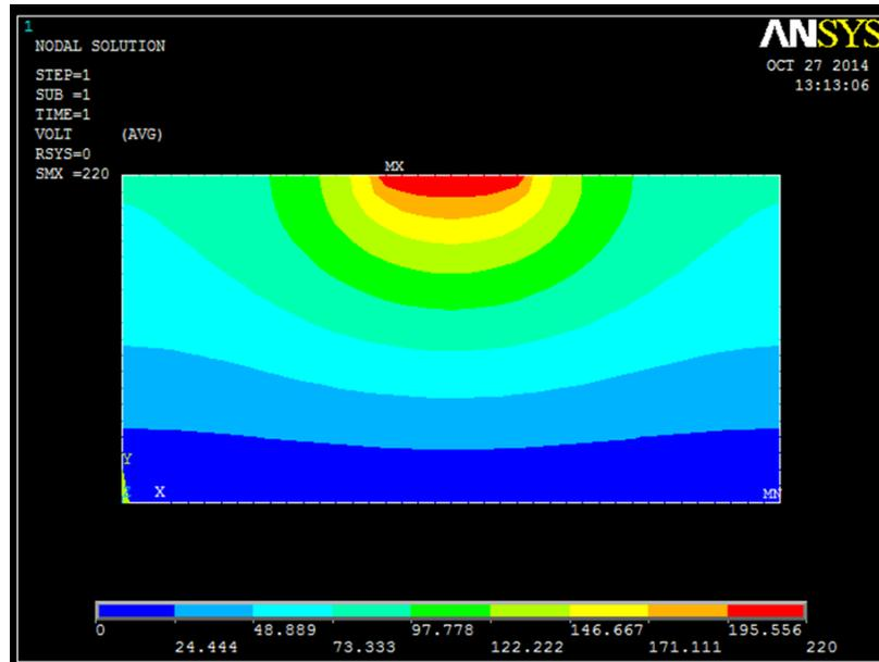
**Fig. 2.** Simulated image of voltage distribution of CFRWCs 11# in the macroscopic field
