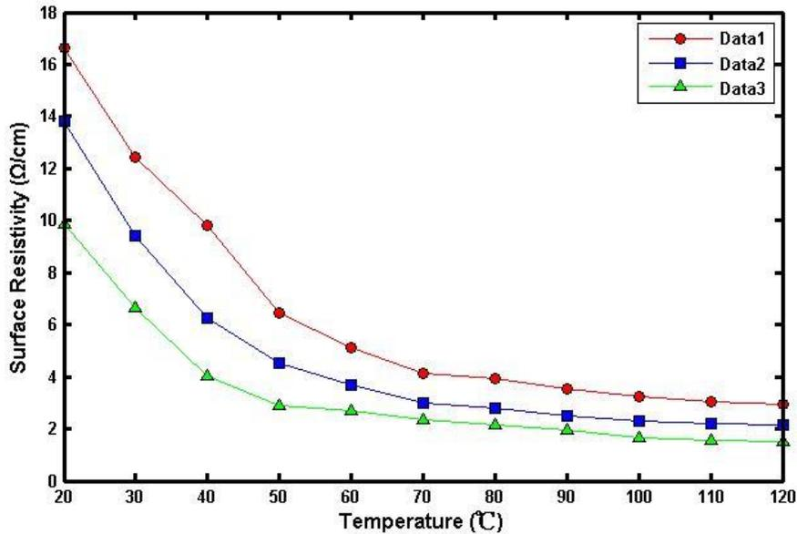
**Fig. 5.** Curves of surface resistivities of single-sided samples of CFRWCs with 55 wt.% (Data 1), 65 wt.% (Data 2), and 75 wt.% (Data 3) carbon fibers
