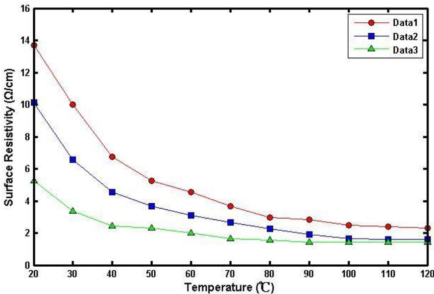
**Fig. 6.** Curves of surface resistivities of two-sided samples of CFRWCs with 55 wt.% (Data 1), 65 wt.% (Data 2), and 75 wt.% (Data 3) carbon fibers
