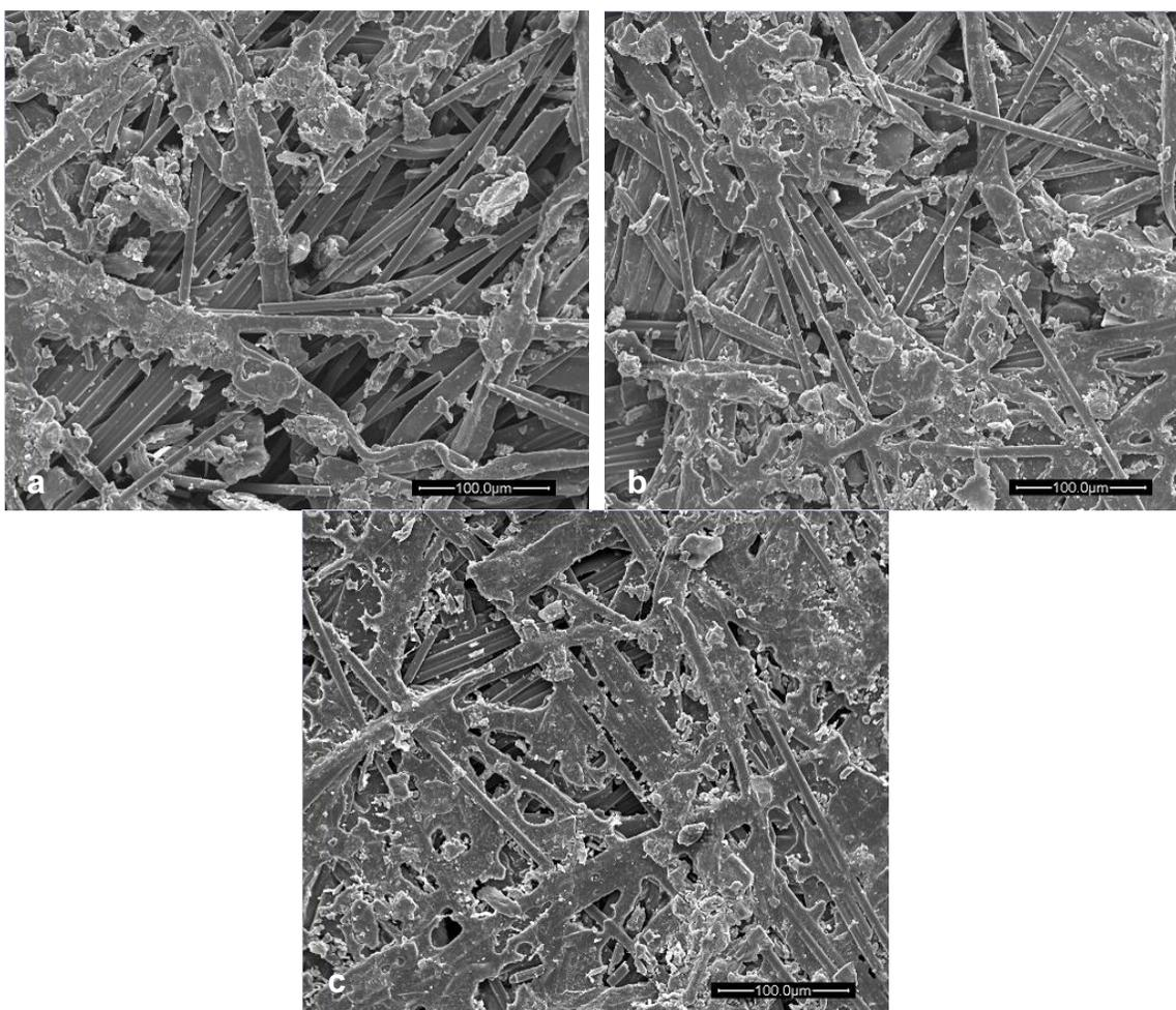
**Fig. 4.** SEM micrographs of CFRWCs samples containing (a) 55 wt.% carbon fibers; (b) 65 wt.% carbon fibers; and (c) 75 wt.% carbon fibers
